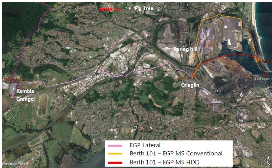
Figure 4-3 Initial concept pipeline and connection options
