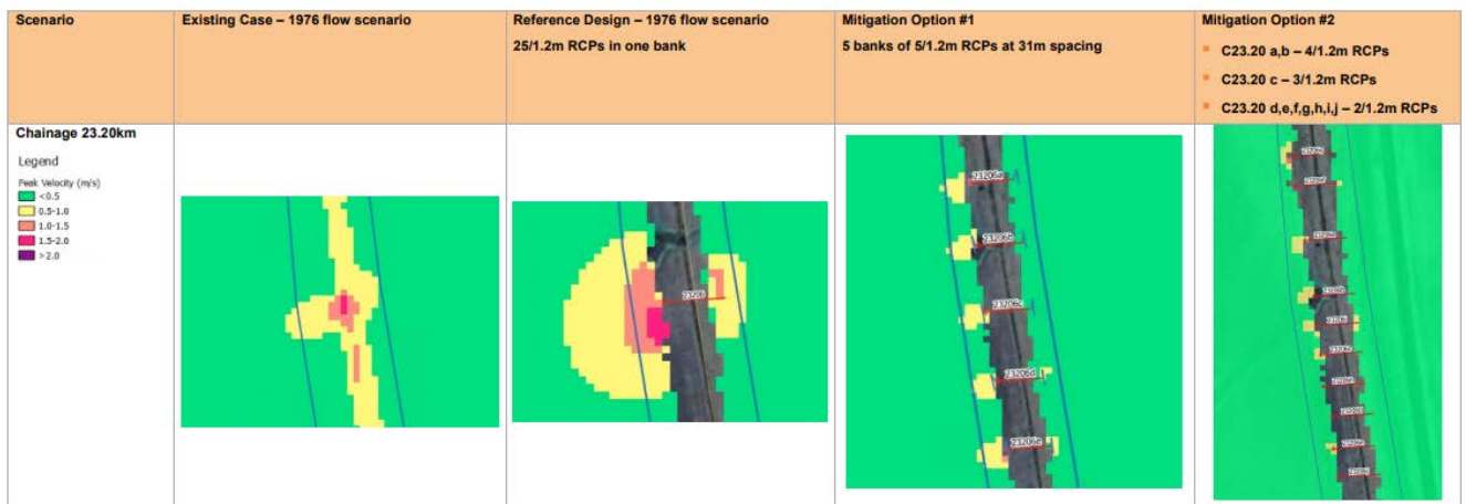
Figure 5 | Example of a culvert design reducing velocity levels on adjoining land (Source: Response to Request for Information Velocity)
