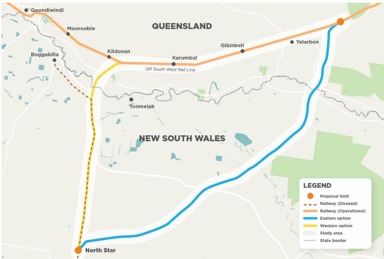
FIGURE 3.1 EASTERN AND WESTERN ALIGNMENT OPTIONS FROM THE ALIGNMENT DEVELOPMENT AND ASSESSMENT REPORT
