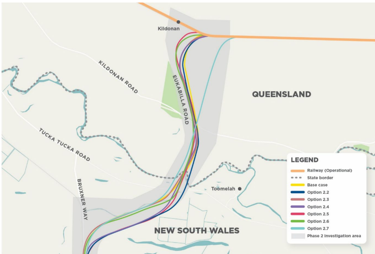
FIGURE 3.4 PHASE 2 ALTERNATIVE GREENFIELD ALIGNMENTS
