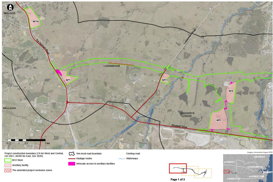
Figure 5-1 Haulage routes and ancillary facility access points
