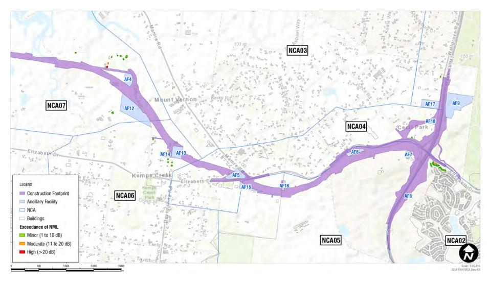
Figure 5-6 Predicted impacts 'scenario 6b, earthworks - typical impact' in all locations (daytime) for the amended project
