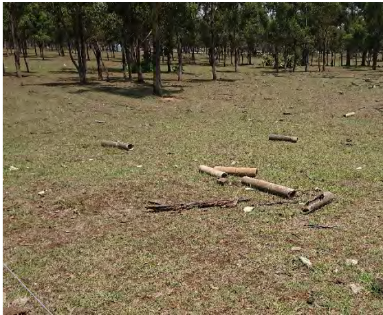
Photograph 3: Sections of potential ACM pipe observed on the surface of existing AEI 21 west of and adjacent to Range Road.
