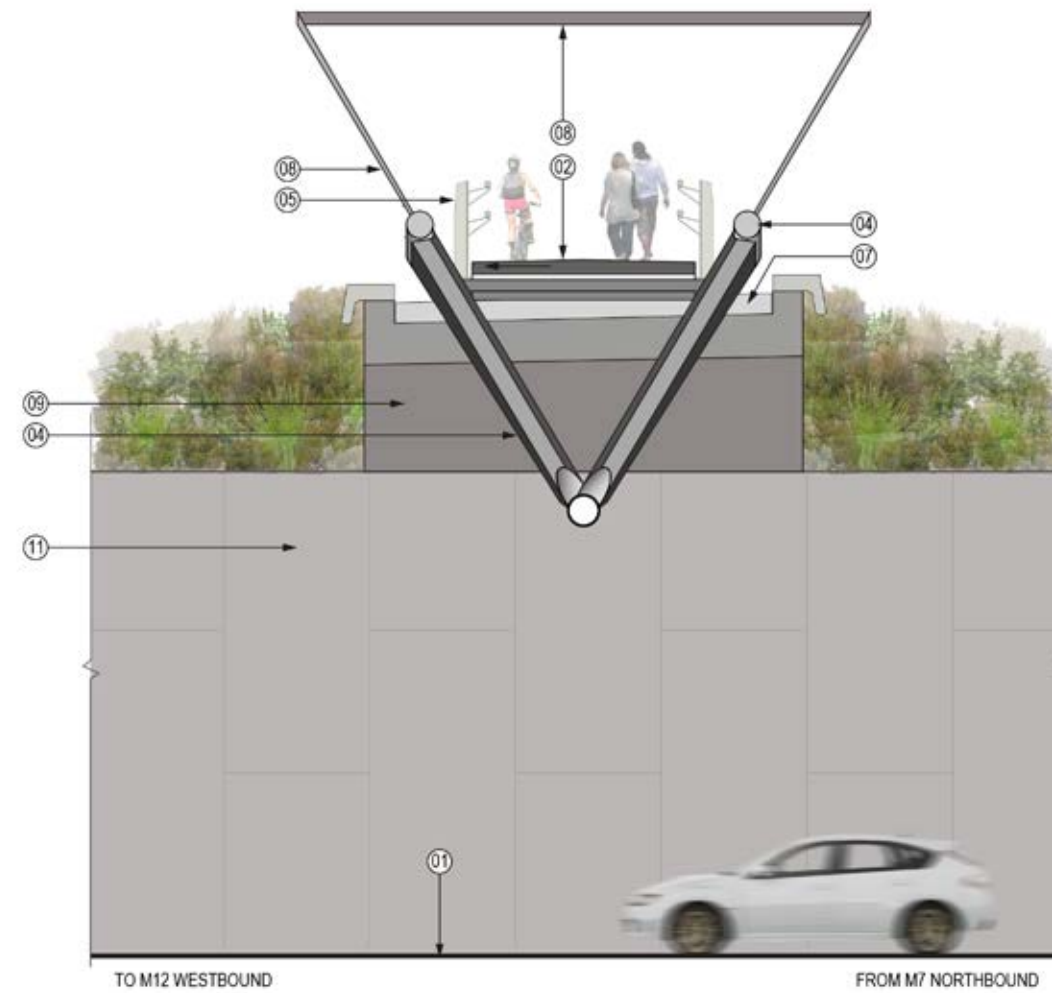
Section - BR16 - Shared user path bridge over M7 Northbound exit ramp
