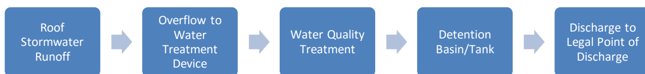
Figure 8: Building Drainage Stormwater Conveyance Flow Chart
