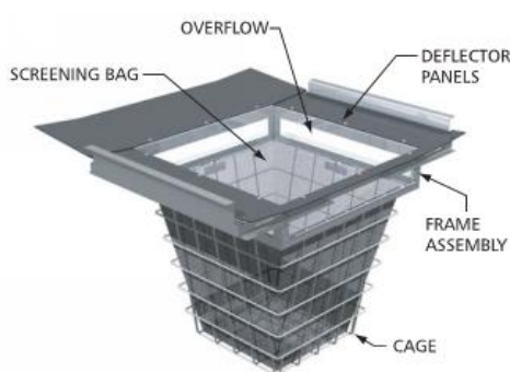
Figure 16: EnviroPod Pit Inlet Trap (Source: Stormwater 360)
