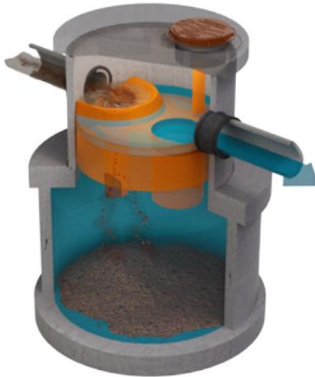
Figure 15: HumesCeptor Unit (Source: Humes)
