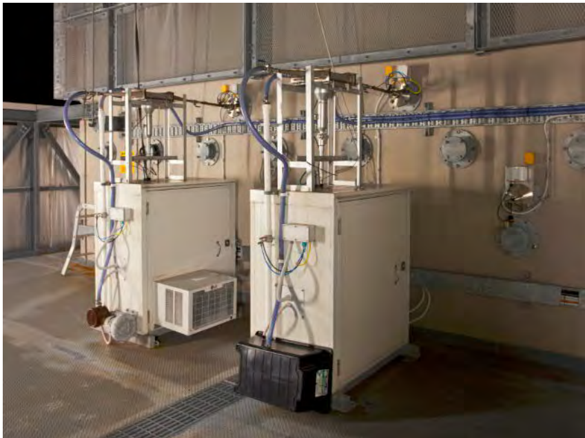
Figure C-6 Air pollution measurements at Lane Cove Tunnel outlet
