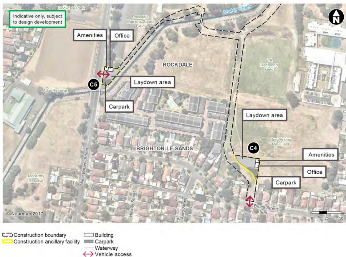
Figure 7-5 Shared cycle and pedestrian pathways construction ancillary facilities (C4 and C5) layout
