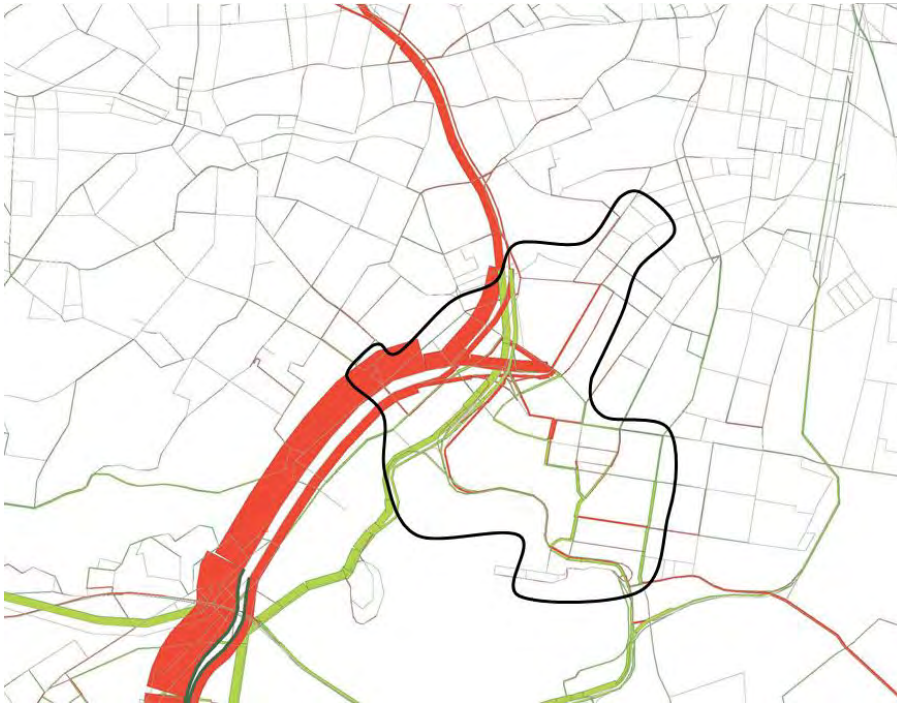
Annexure Figure 3 St Peters interchange: comparison of 2036 AM peak hour volumes ‘do something’ and ‘do minimum’
