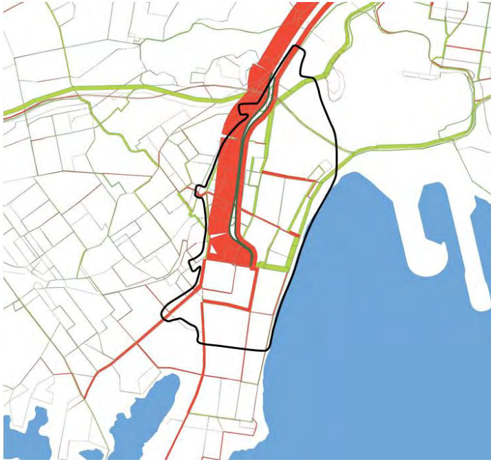
Annexure Figure 1 President Avenue intersection: comparison of 2036 AM peak hour volumes 'do something' and 'do minimum'
