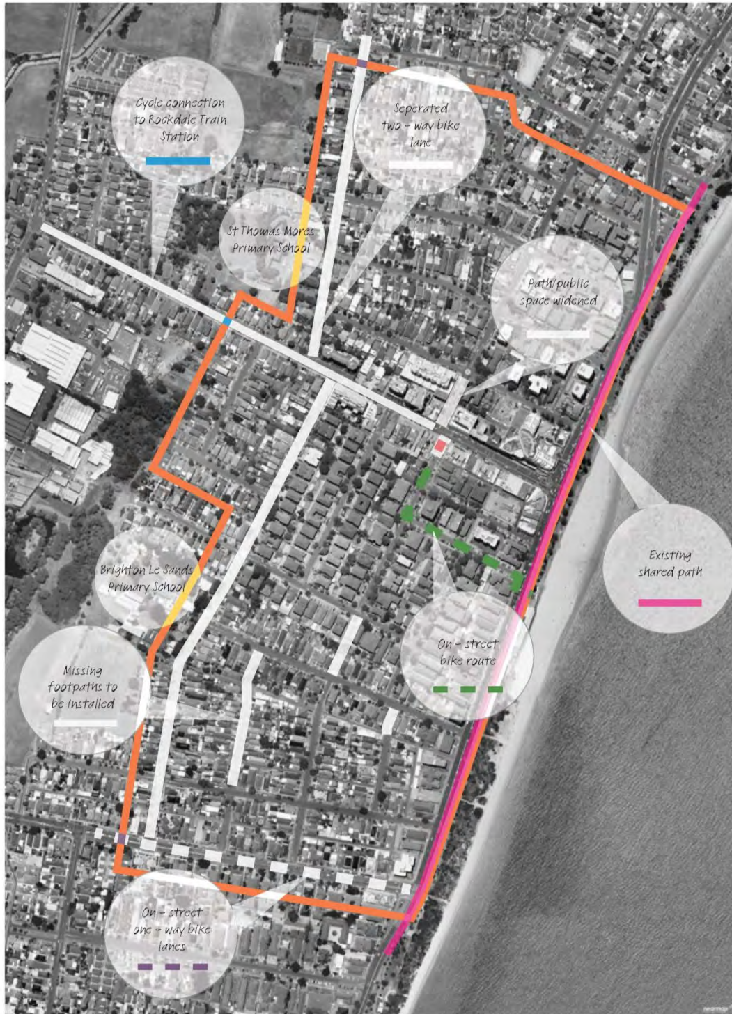
Figure 8-8 Brighton-Le-Sands: Recommended pedestrian path upgrades and cycle path network
