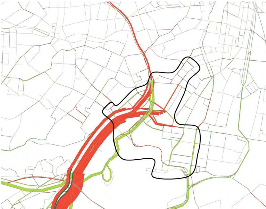
Annexure Figure 4 St Peters interchange: comparison of 2036 PM peak hour volumes ‘do something’ and ‘do minimum’
