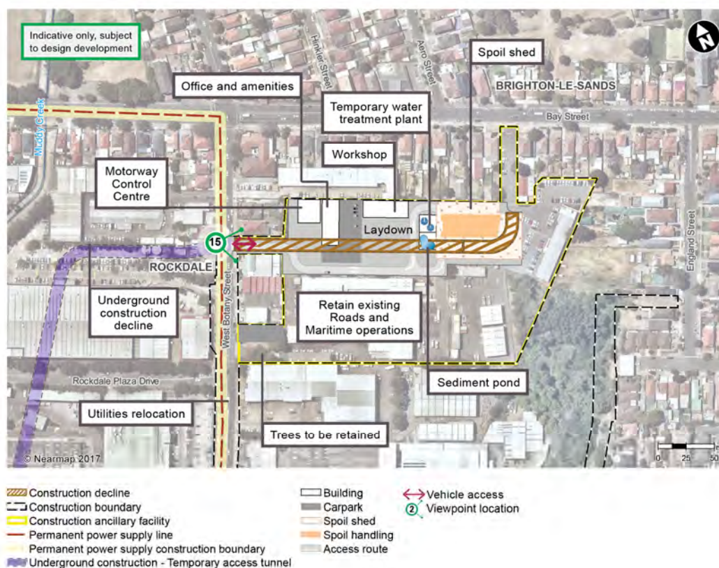
Figure 8-21 Rockdale Motorway Control Centre layout during construction (Rockdale construction ancillary facility – C2)
