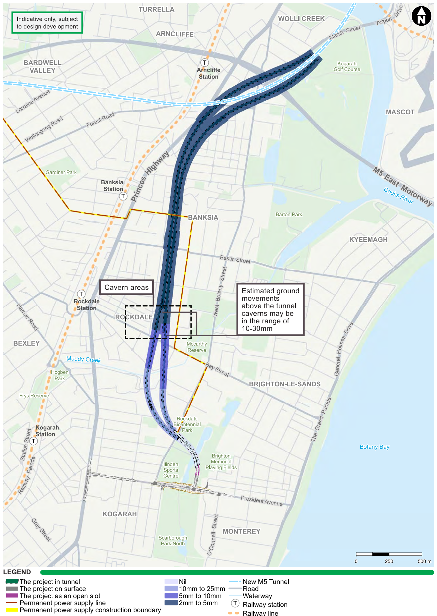
Figure 17-7 Preliminary indicative ground movements as a result of the project
