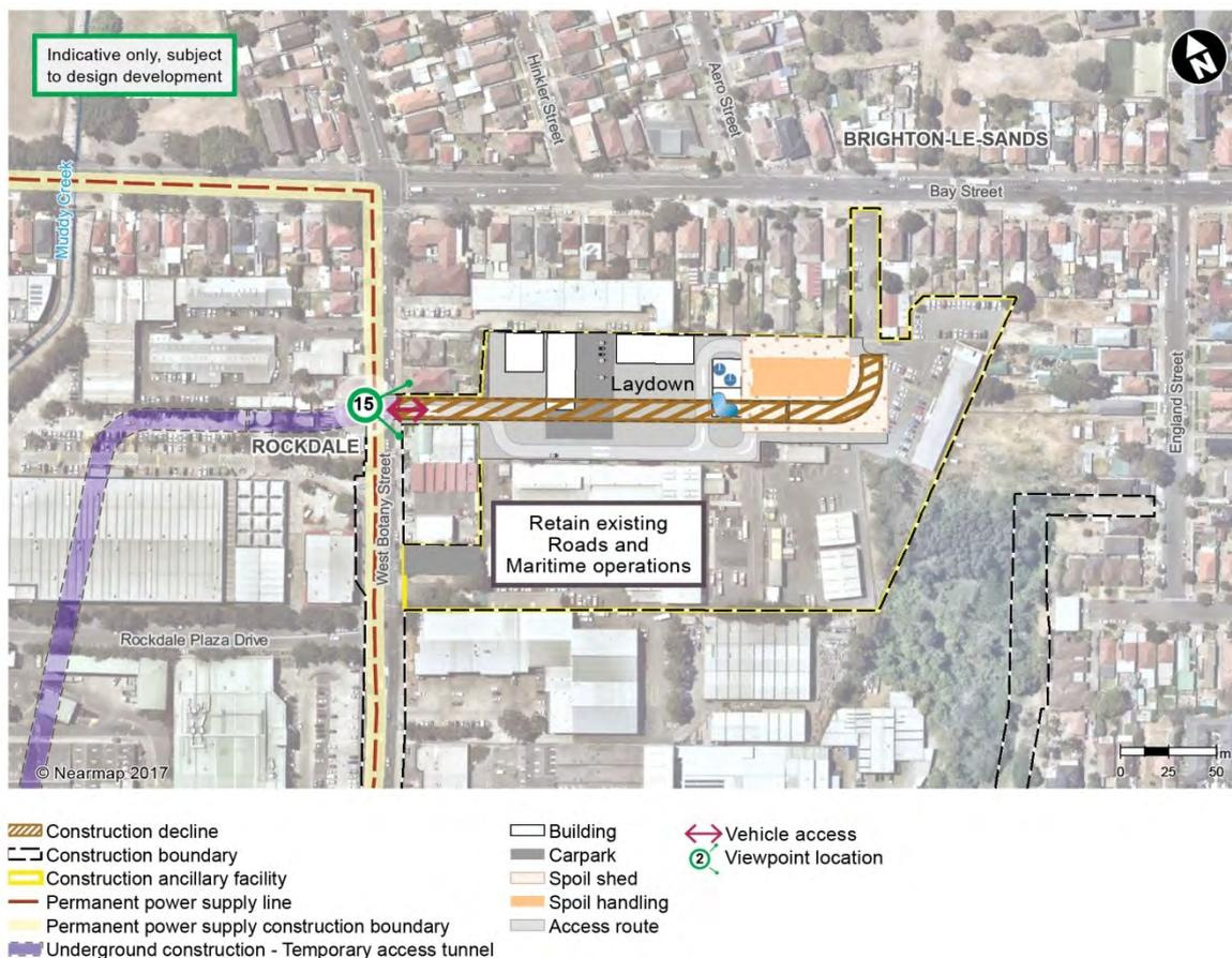
**Figure 13-38 Construction layout and viewpoint locations, southern surface works (President Avenue) - Rockdale construction ancillary facility (C2)**
