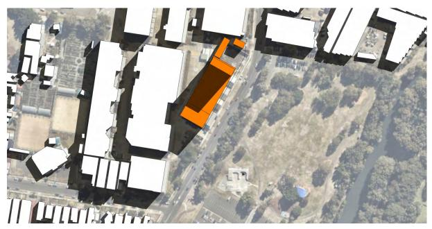
Figure 13-50 Overshadowing diagram - MOC3 - June 21 at 3:00pm (winter solace)
