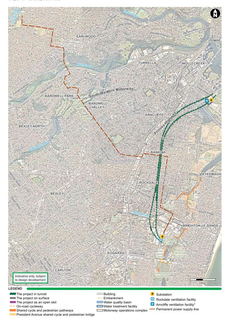
Figure 13-16 Permanent power supply
