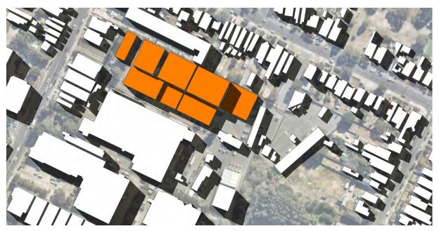
Figure 13-47 Overshadowing diagram – MOC2 – June 21 at 9:00am (winter solace)
