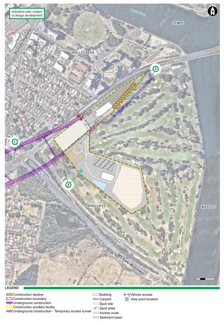
Figure 13-37 Construction layout and viewpoint locations, northern surface works - Arncliffe construction ancillary facility (C1)
