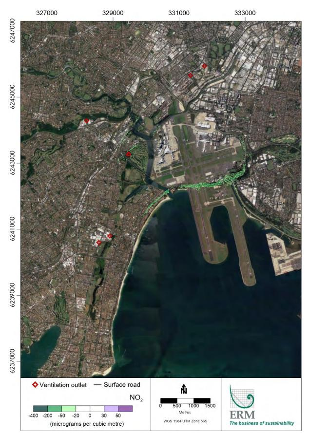
Figure 9-55 Contour plot of change in maximum one-hour mean  $NO_2$  concentration in the 2036 cumulative scenario (all sources, 2036-DSC minus 2036-DM)
