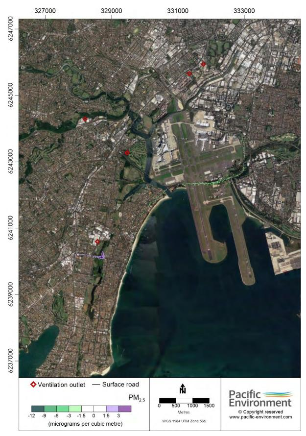
Figure 9-38 Contour plot of change in maximum 24-hour mean PM<sub>2.5</sub> concentration in 2036 Do Something scenario (all sources, 2036-DS minus 2036-DM)
