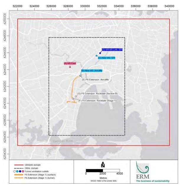
Figure 9-4 Modelling domains for GRAMM and GRAL (grid system MGA94) showing the ventilation outlets included in the air quality assessment.
