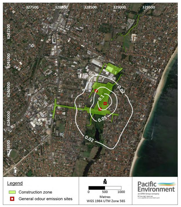
Figure 9-10 Predicted 99th percentile H<sub>2</sub>S concentration due to exposure of acid sulfate material ( $\mu$ g/m<sup>3</sup>)
