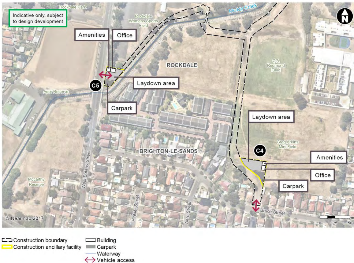
Figure 7-6 Shared cycle and pedestrian pathways construction ancillary facilities (C4 and C5) indicative layout
