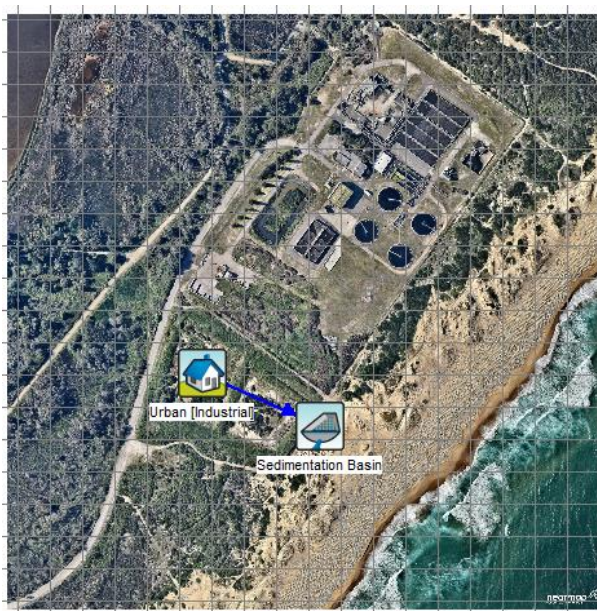
Figure 2 MUSIC model for the Desalination Plant
