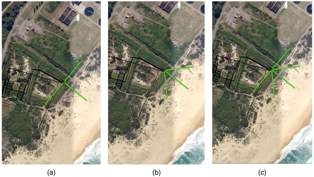
Figure 5-4 Intake design: a) three perpendicular; b) three diagonal; c) five diagonal and perpendicular
