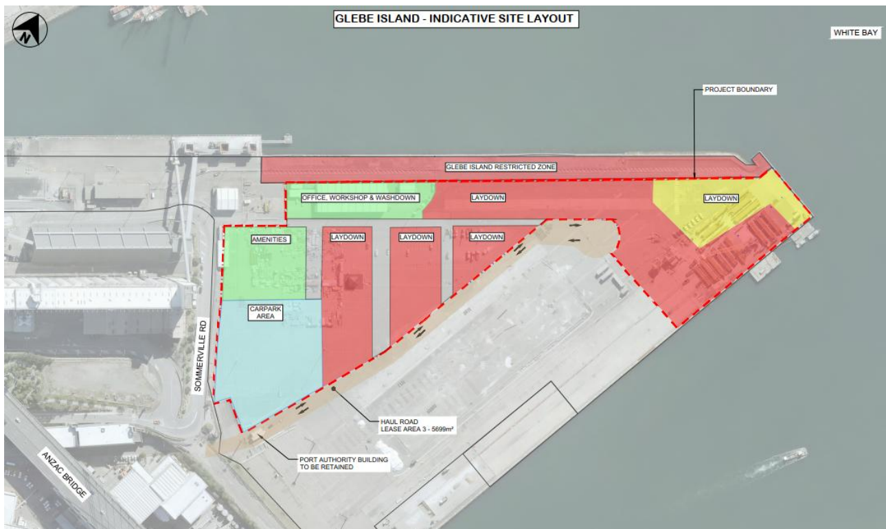
Figure 1 Glebe Island construction support site layout and parking
