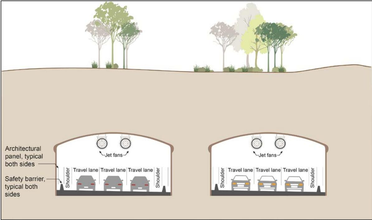
Figure 9 | Cross section of Mainline Tunnels (Source: EIS)
