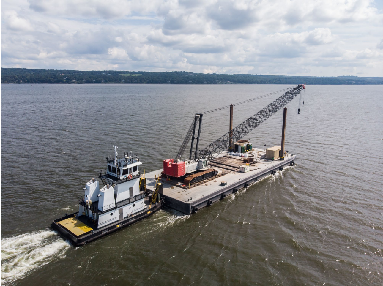
Figure 6-12 Example of a flat top work barge and cofferdam
