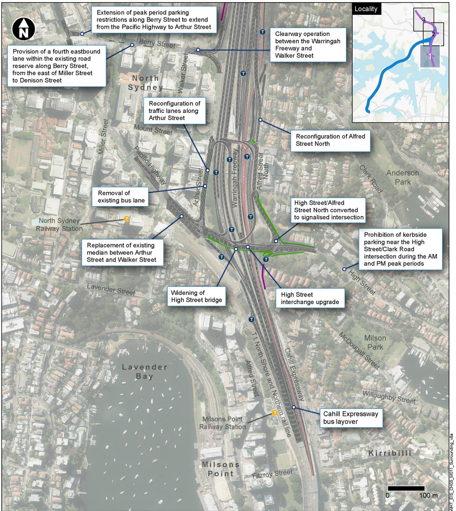
**Figure 5-30 Upgrades and changes to the surrounding road network of the Warringah Freeway Upgrade component (map 1)**
