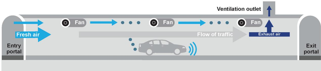
**Figure 5-15 Tunnel air flow during normal operating conditions**
