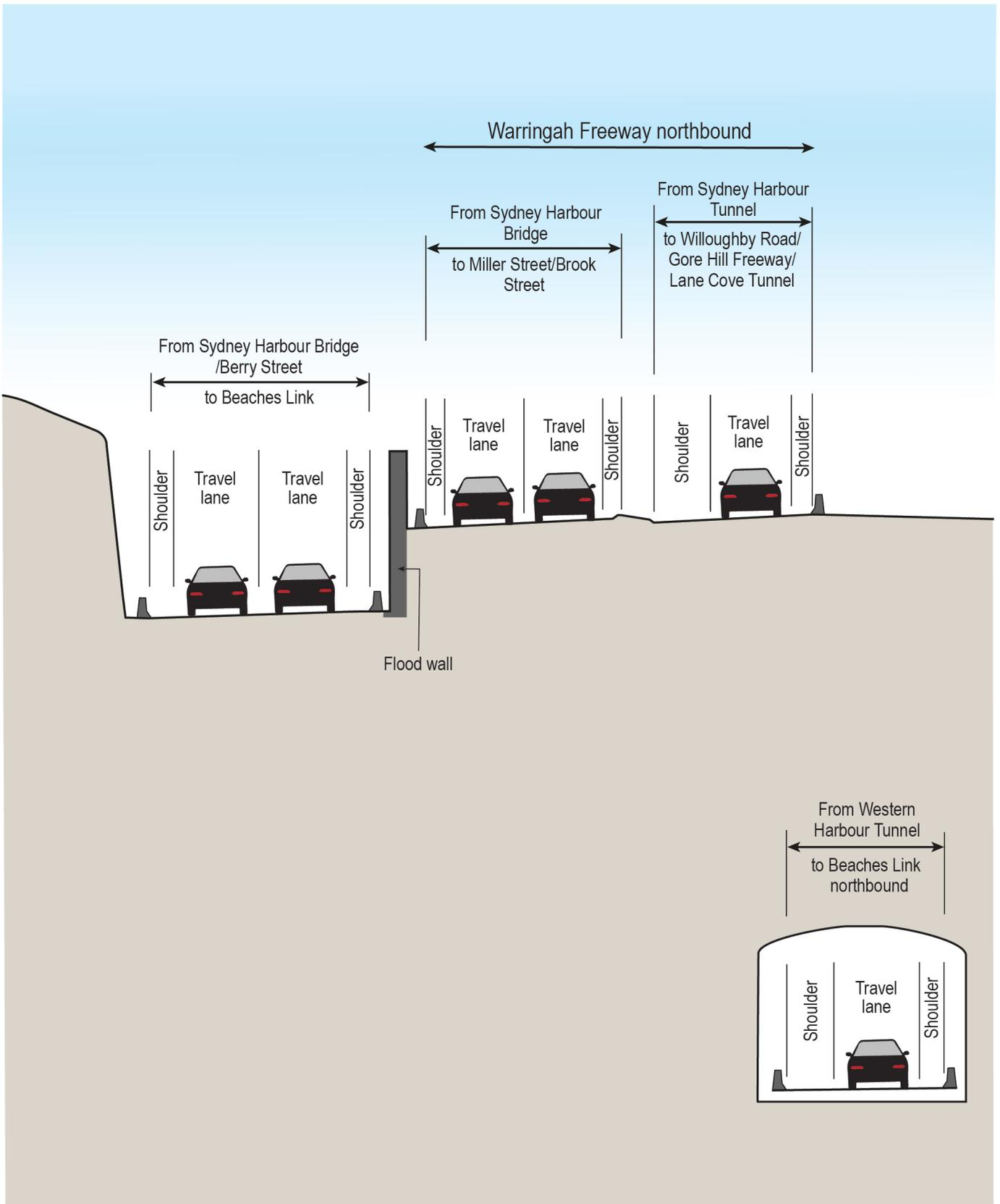
**Figure 5-23 Indicative cross-section through the connection between the Beaches Link and Gore Hill Freeway Connection project and the Warringah Freeway Upgrade (part 1)**
