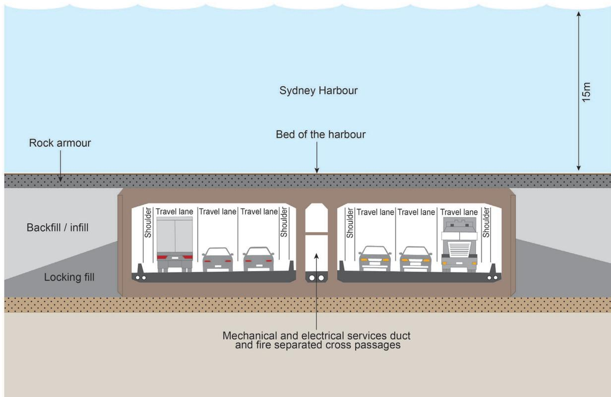
**Figure 5-11 Indicative cross-section of the middle sections of immersed tube tunnels (Sydney Harbour)**
