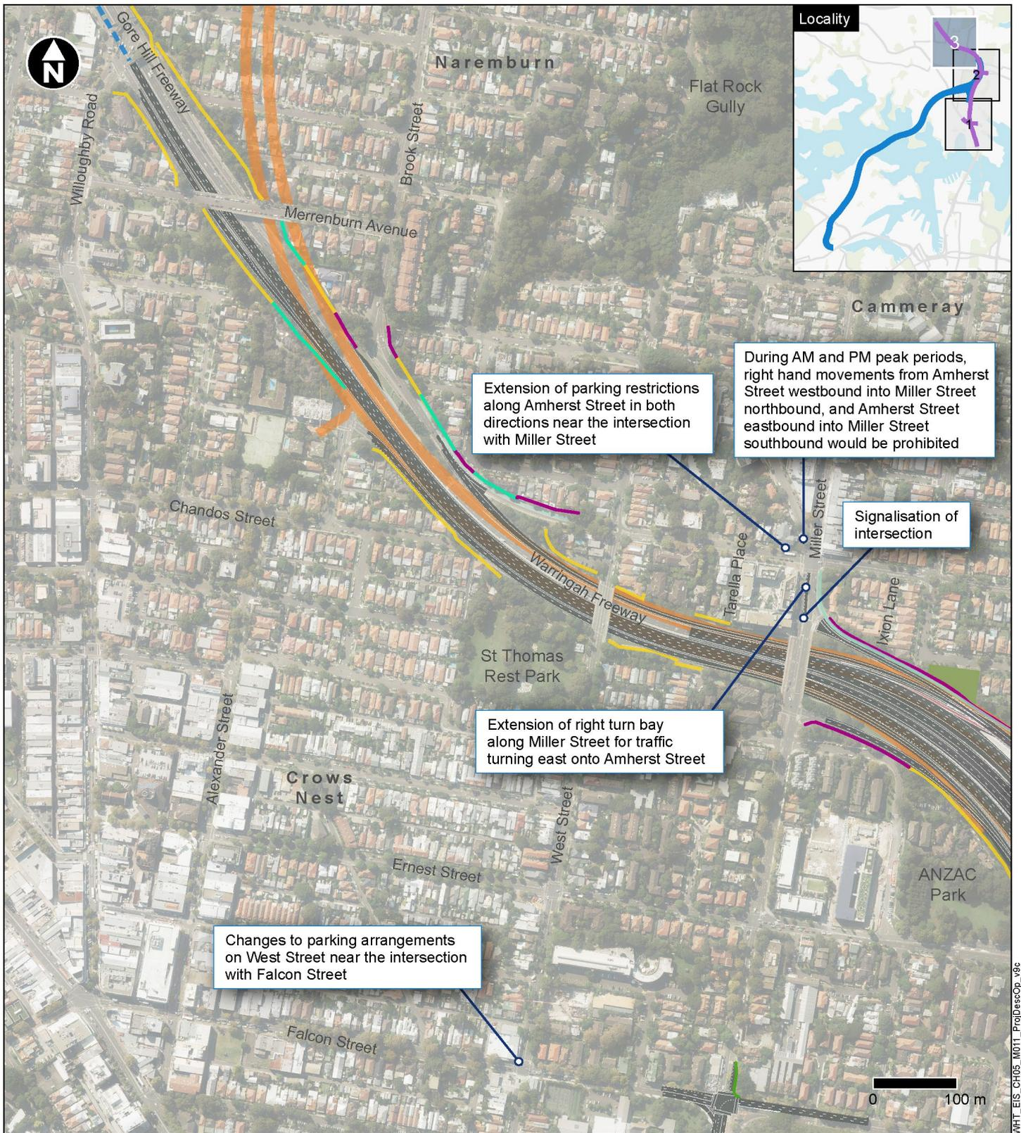
**Figure 5-32 Upgrades and changes to the surrounding road network of the Warringah Freeway Upgrade component (map 3)**
