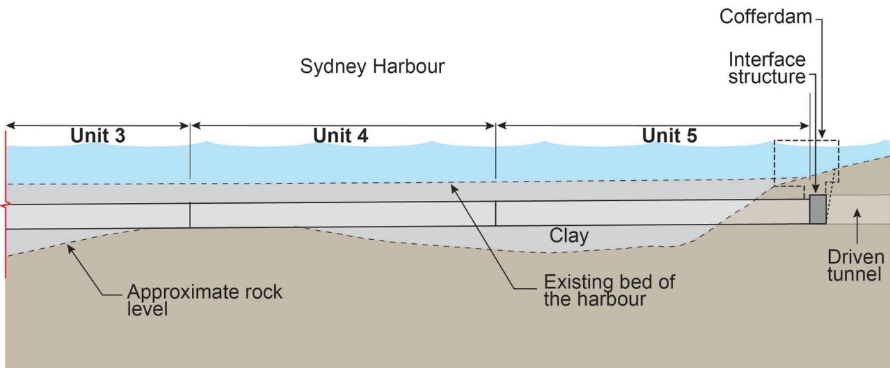
**Figure 5-9** Indicative long section of the immersed tube tunnel crossing of Sydney Harbour
