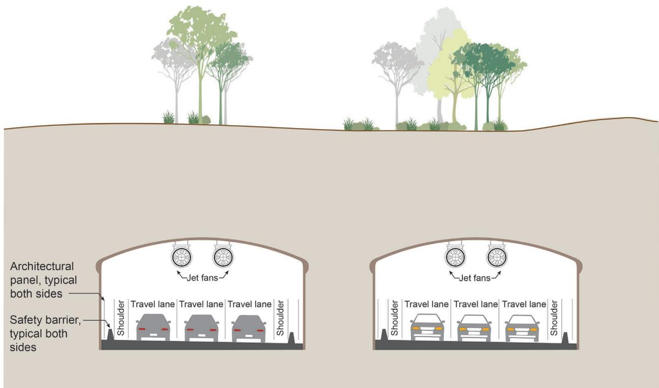
**Figure 5-8** Indicative cross-section of the driven mainline tunnels
