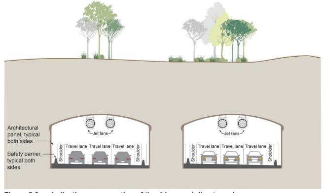
Figure 5-8 Indicative cross-section of the driven mainline tunnels
