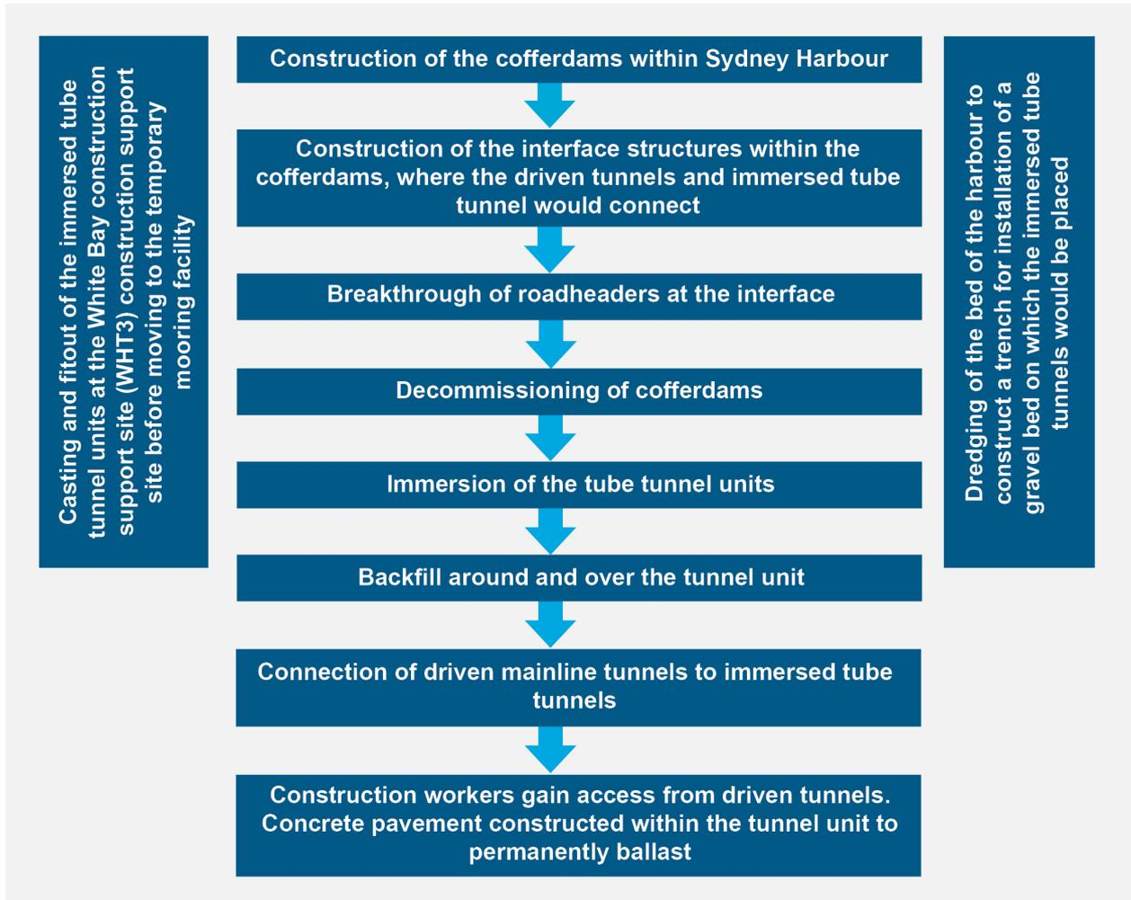
Figure 6-10 Indicative construction process for the immersed tube tunnels
