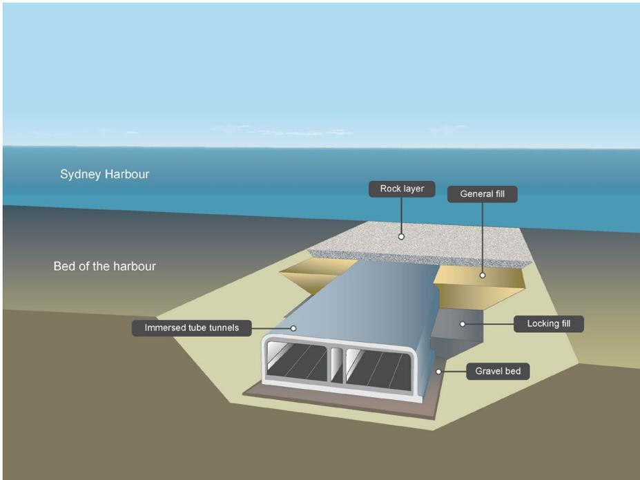
**Figure 6-18 Example of an immersed tube tunnel**
