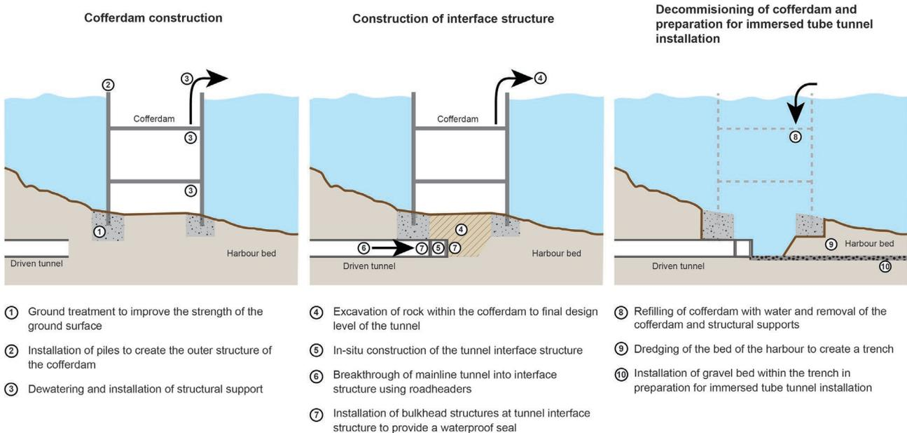
**Figure 6-13 Indicative process for constructing the tunnel interface structures**
