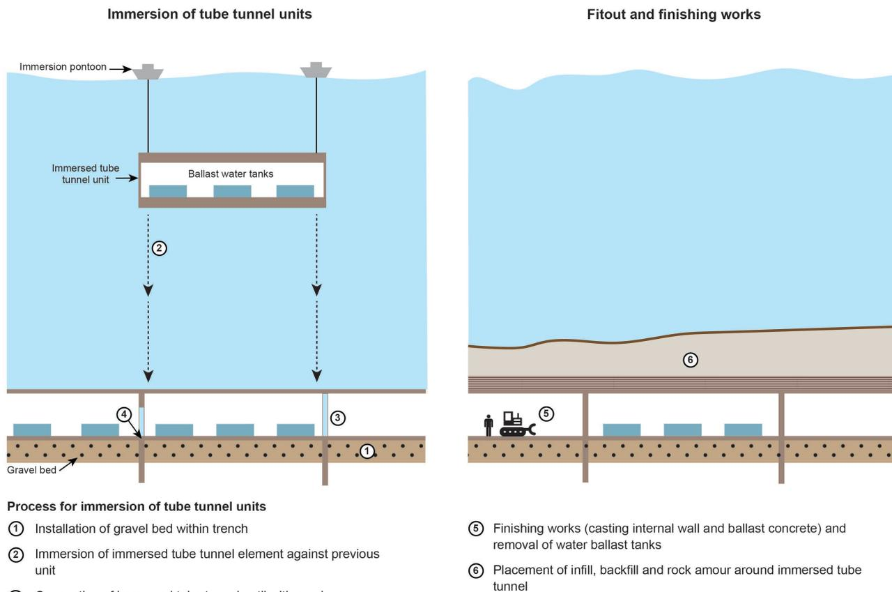
**Figure 6-19 Indicative immersed tube tunnel installation sequence**
