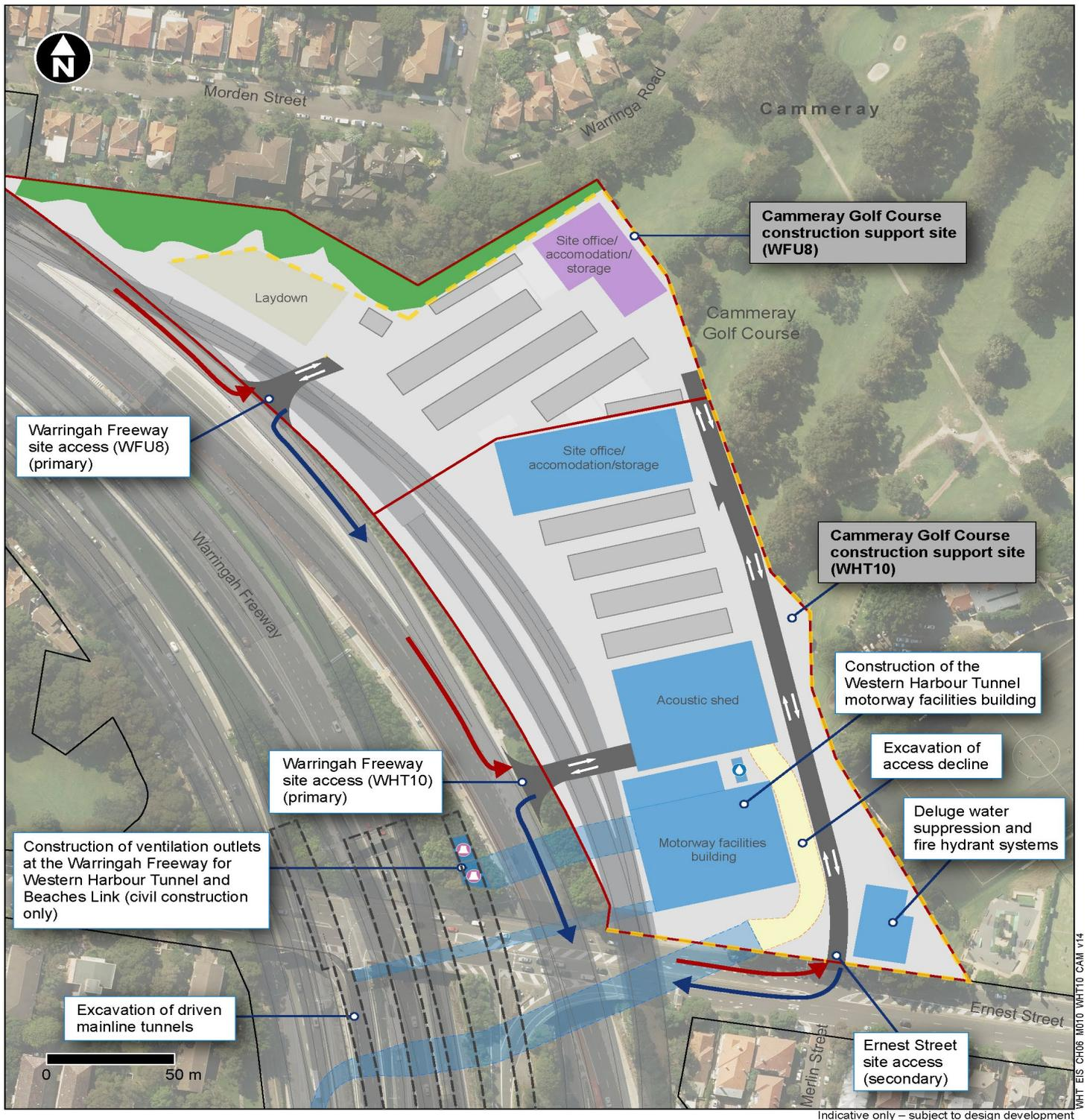
**Figure 6-34 Indicative layout – Cammeray Golf Course construction support site**
