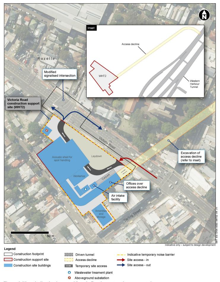
Figure 6-27 Indicative layout – Victoria Road construction support site
