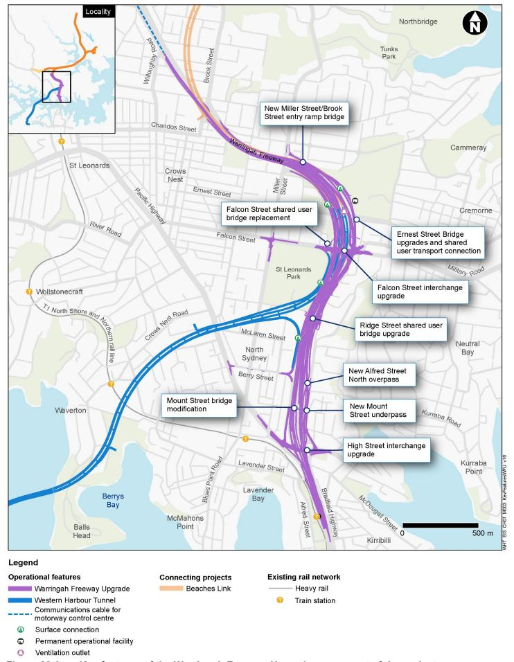
Figure 28-3 Key features of the Warringah Freeway Upgrade component of the project
