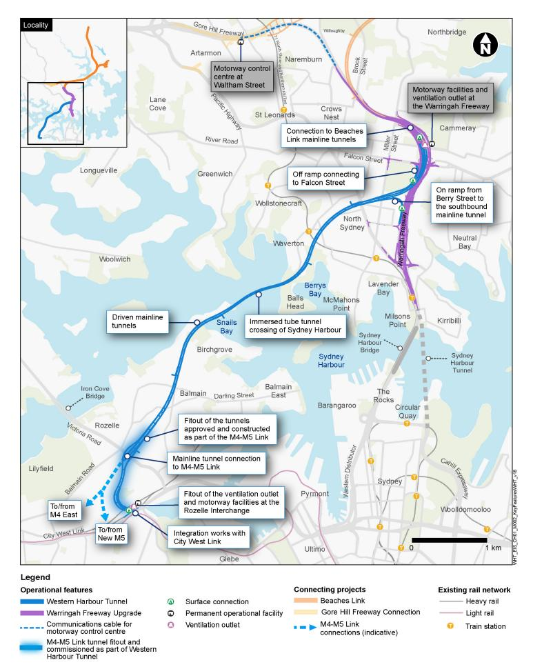
Figure 28-2 Key features of the Western Harbour Tunnel component of the project
