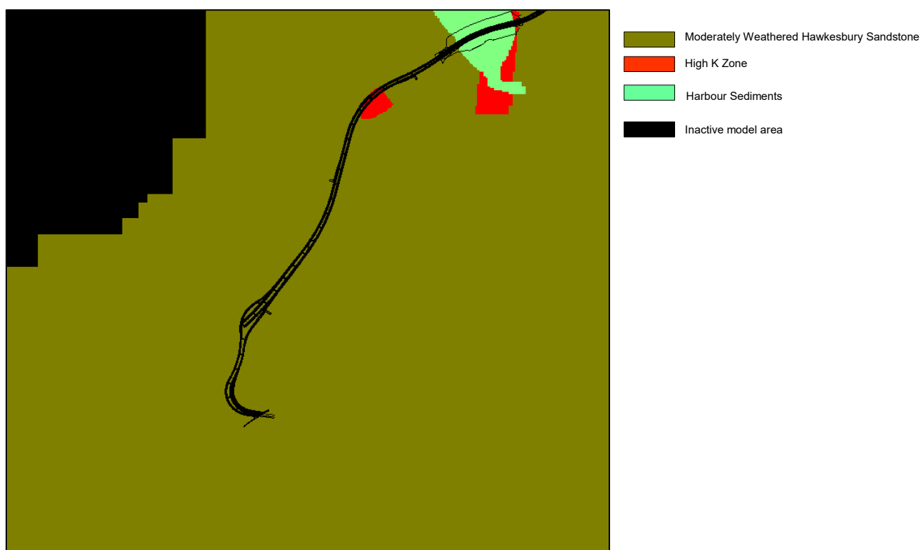
Figure 3-5: Hydrostratigraphic units in Layer 2 – South Model
