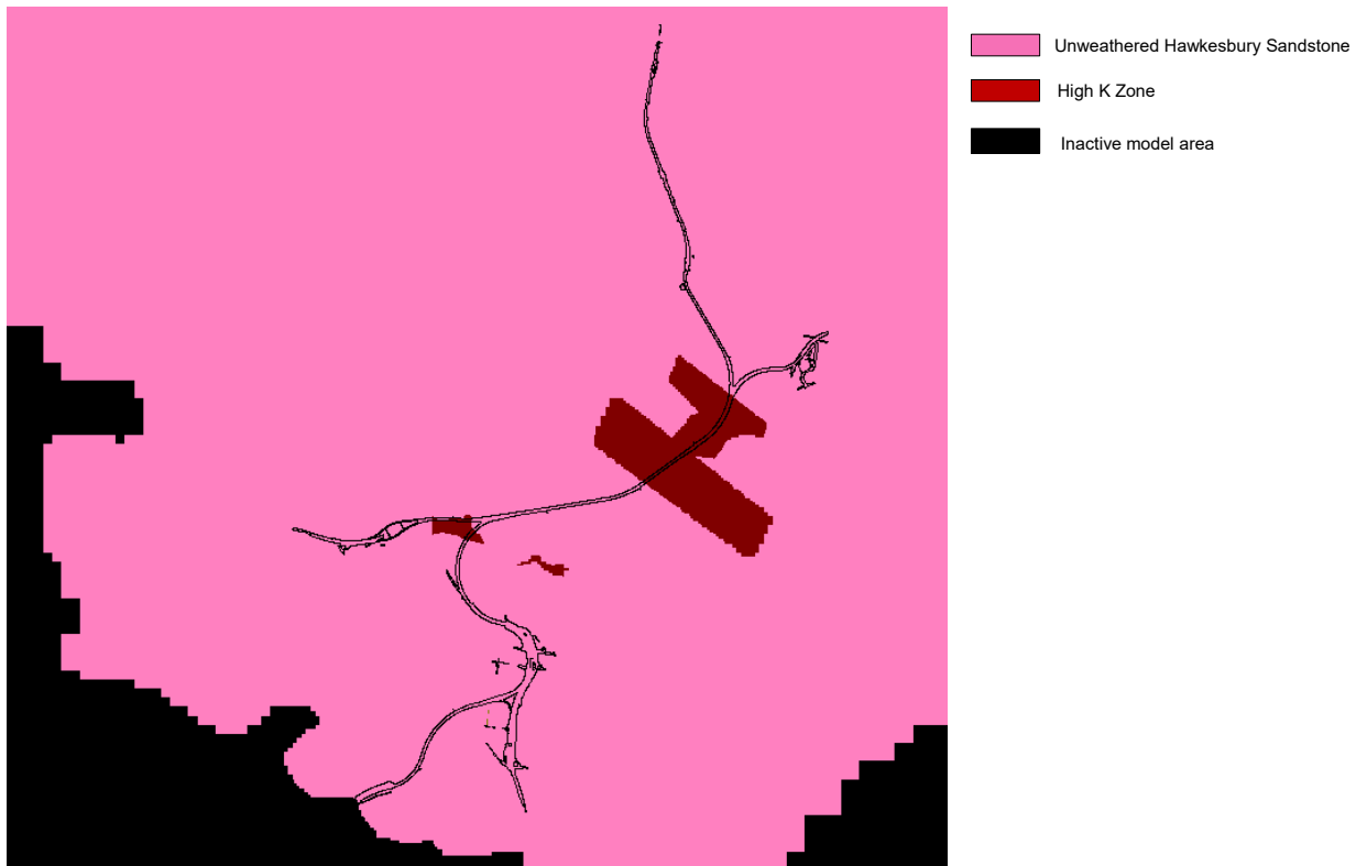
Figure 3-14: Hydrostratigraphic units in Layer 5 to Layer 7 – North Model.
