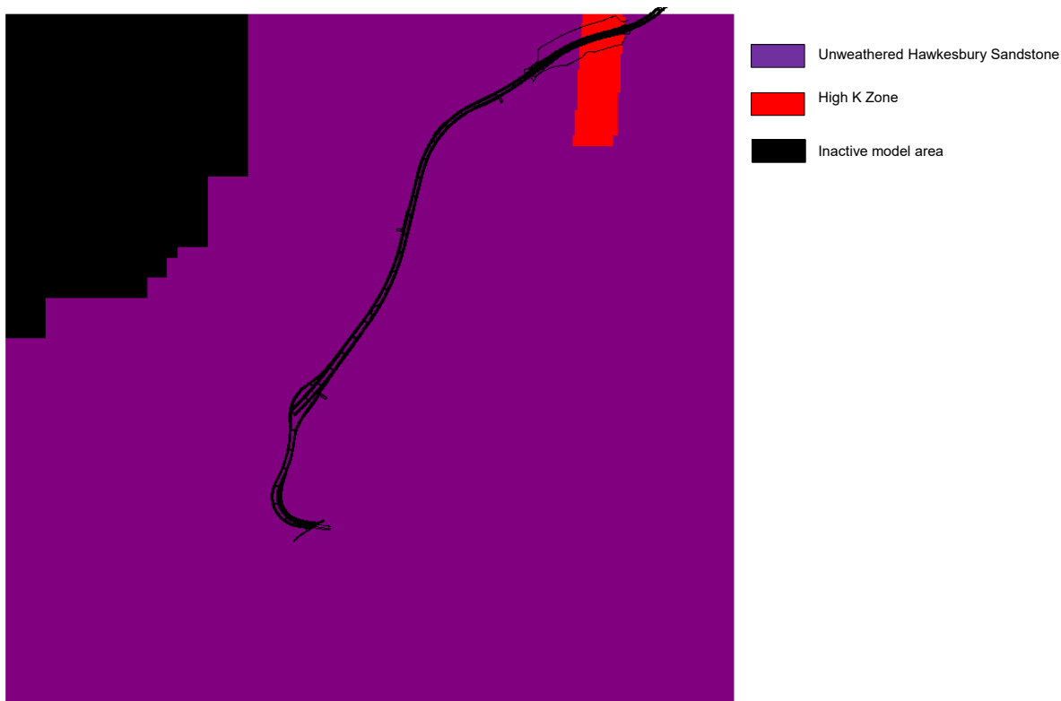
Figure 3-8: Hydrostratigraphic units in Layer 5 to 7 – South Model
