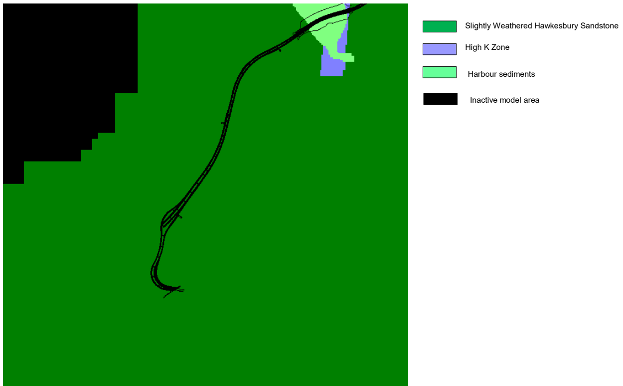
Figure 3-7: Hydrostratigraphic units in Layer 4 - South Model
