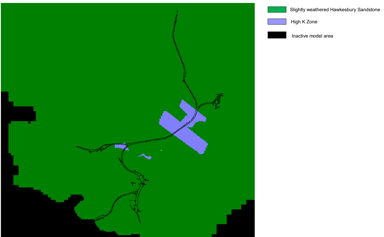
Figure 3-13: Hydrostratigraphic Units in Layer 4 – North Model
