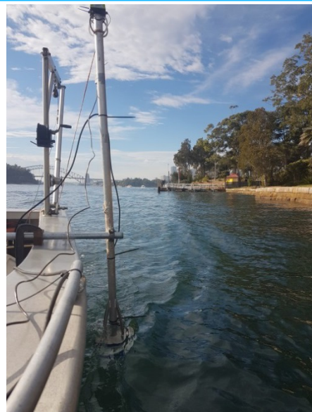
Vessel-mounted ADCP transect setup
