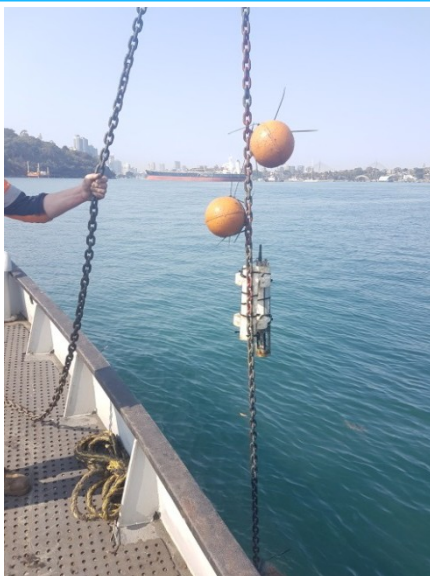
Water quality sonde during deployment at WH2
