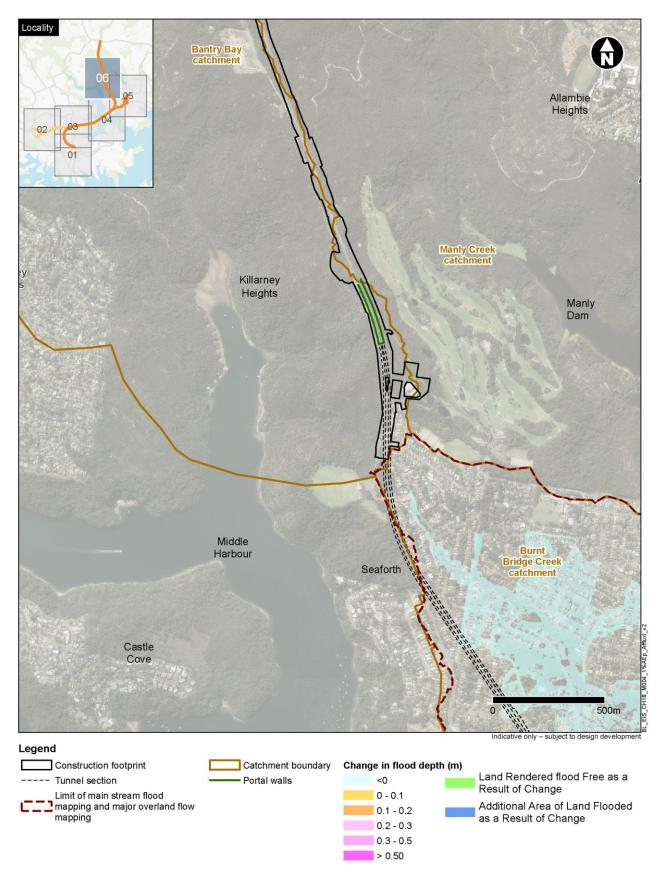
Figure 18-20 Change in flood depth under operational conditions – 1% AEP event (map 6)
