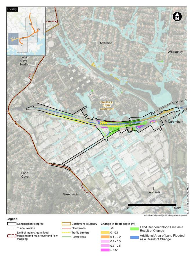
Figure 18-16 Change in flood depth under operational conditions – 1% AEP event (map 2)
