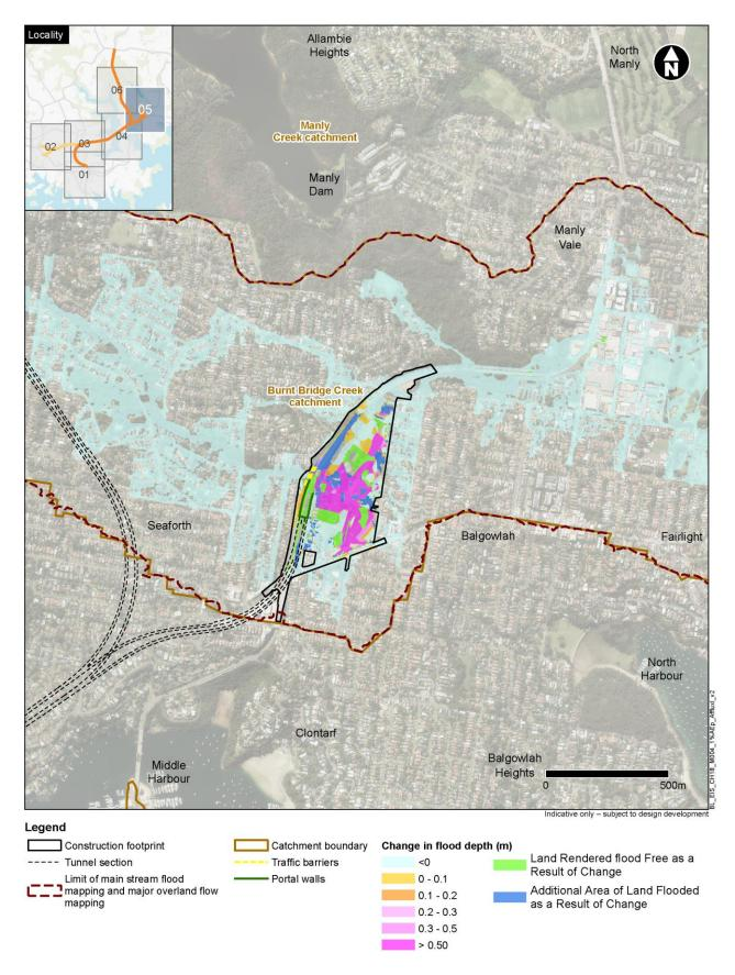
Figure 18-19 Change in flood depth under operational conditions – 1% AEP event (map 5)
