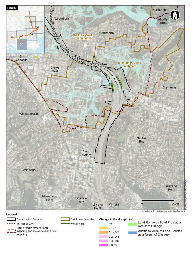
Figure 18-15 Change in flood depth under operational conditions – 1% AEP event (map 1)
