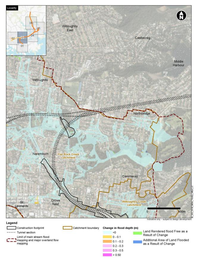
Figure 18-17 Change in flood depth under operational conditions – 1% AEP event (map 3)
