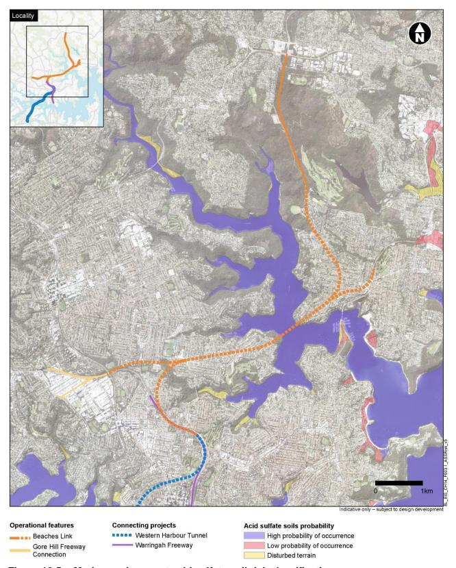
Figure 16-5 Marine environment acid sulfate soil risk classification
