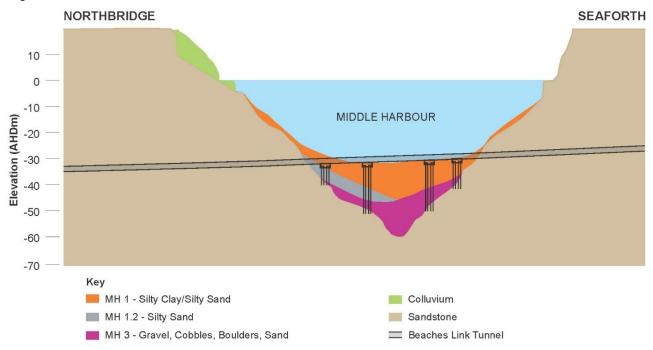
Figure 16-3 Middle Harbour marine sediment and geology profile
