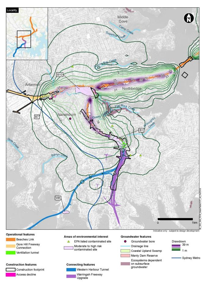
Figure 16-13 Groundwater drawdown contours for the project during operation in 2128 – South of Middle Harbour
