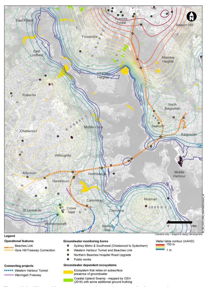
Figure 16-6 Water table contour map and groundwater monitoring network
