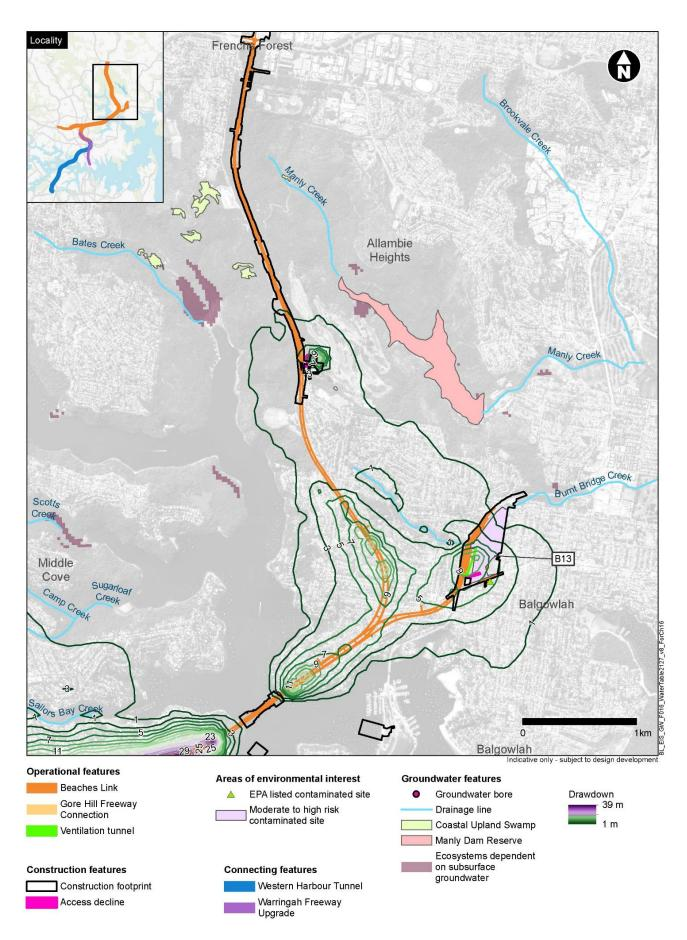
Figure 16-14 Groundwater drawdown contours for the project during operation in 2128 – North of Middle Harbour
