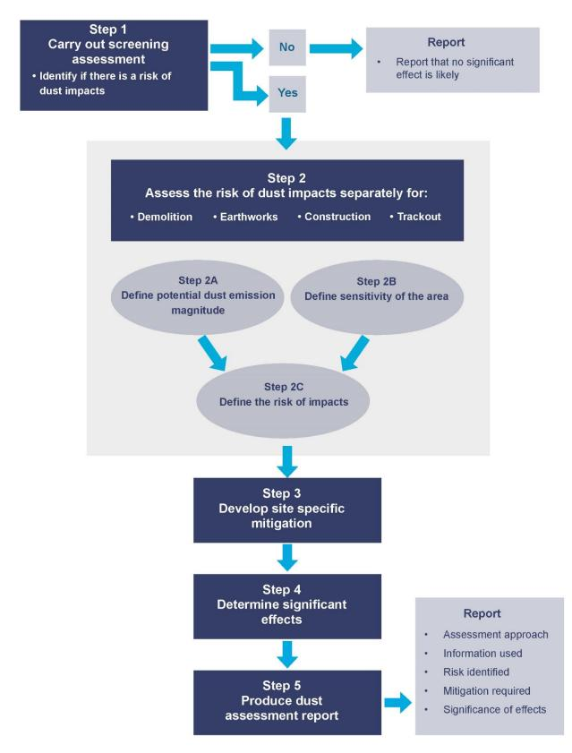
Figure 12-1 Construction dust assessment procedure (IAQM, 2014)
