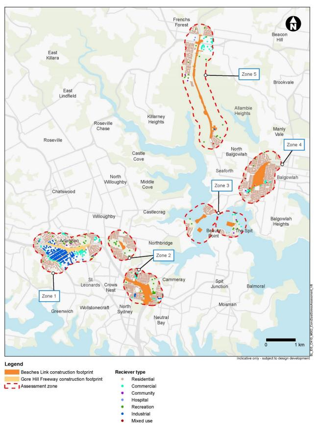
Figure 12-4 Construction dust screening assessment – receivers near the construction footprint
