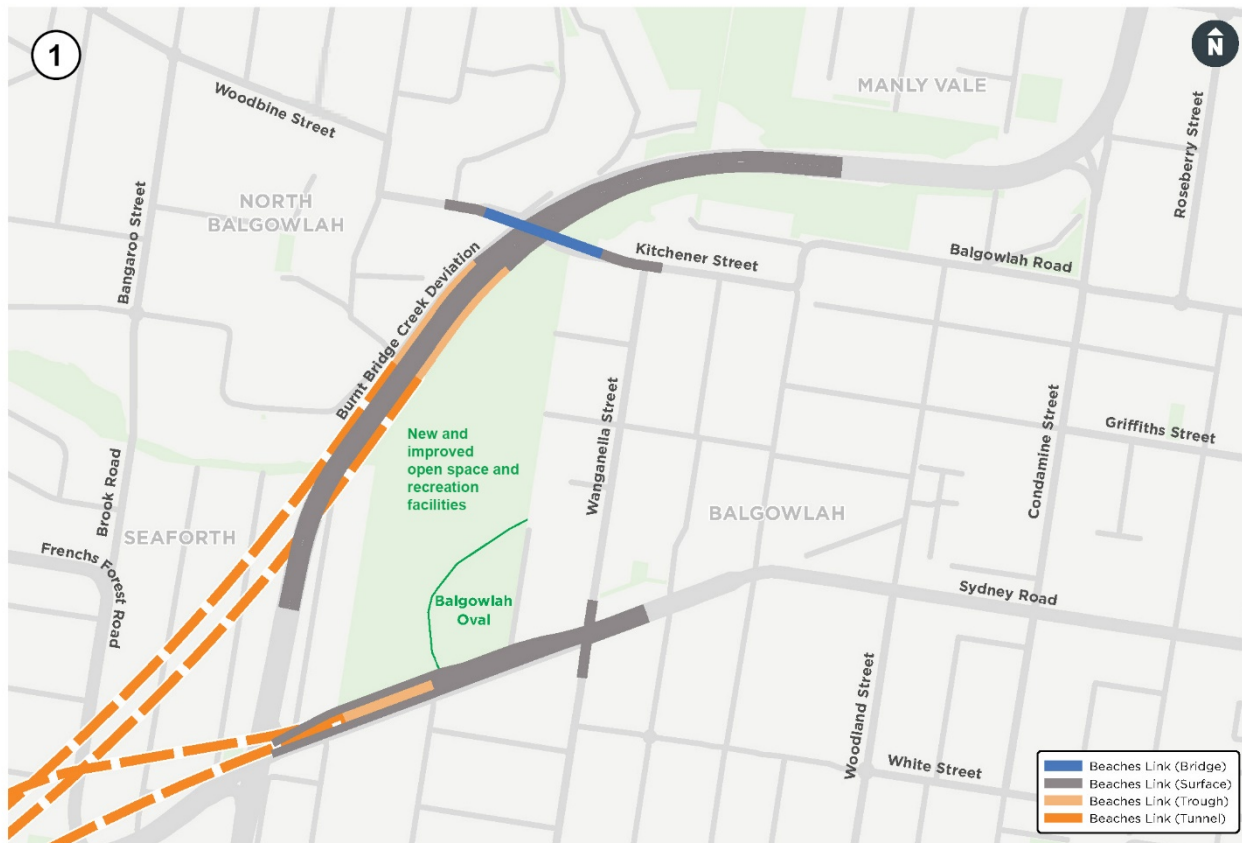
Figure 4-22 Alternative 1 – Ramps emerging in Sydney Road
