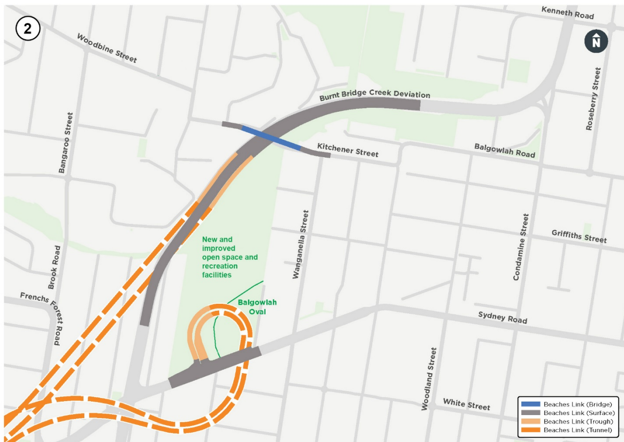
Figure 4-23 Alternative 2 - Tunnel loop ramps to Sydney Road
