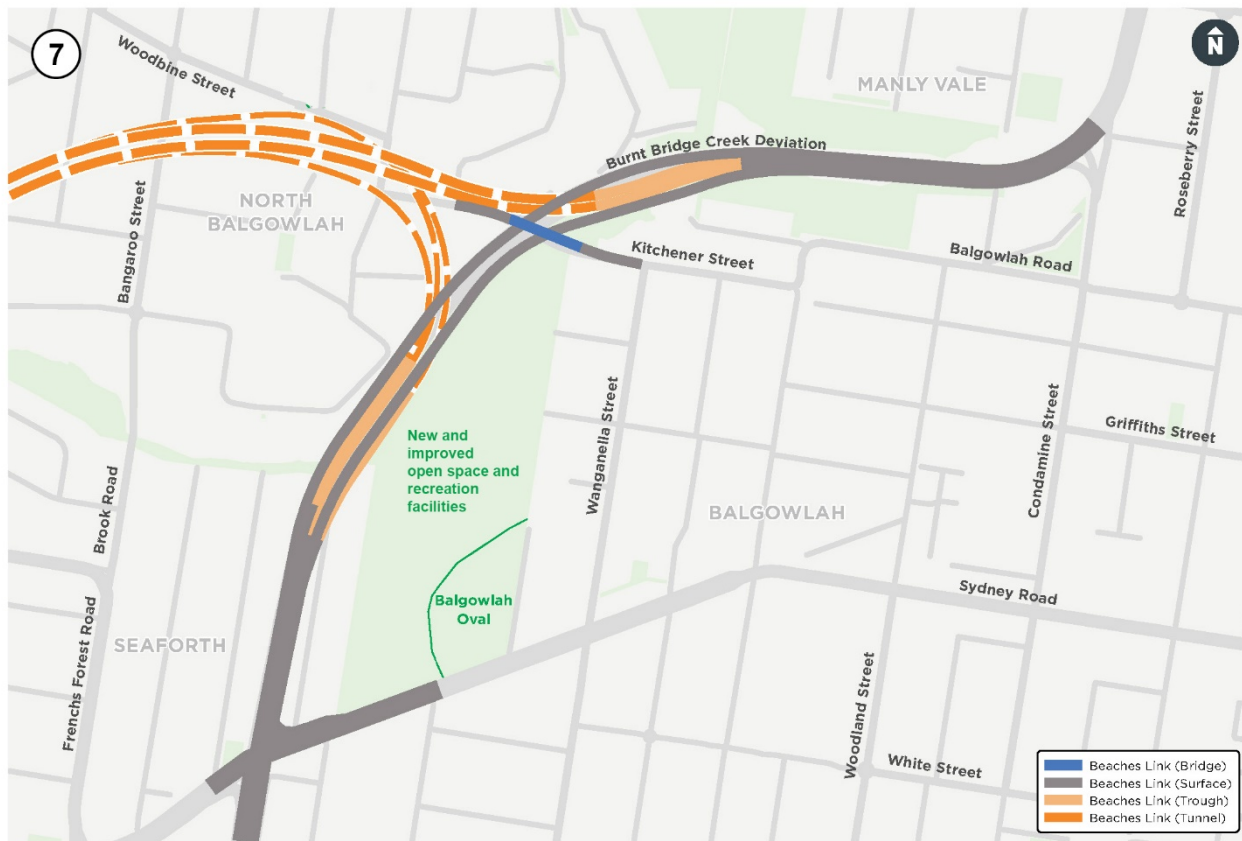
Figure 4-30 Alternative 7 - North and south facing tunnel ramps to Burnt Bridge Creek Deviation
