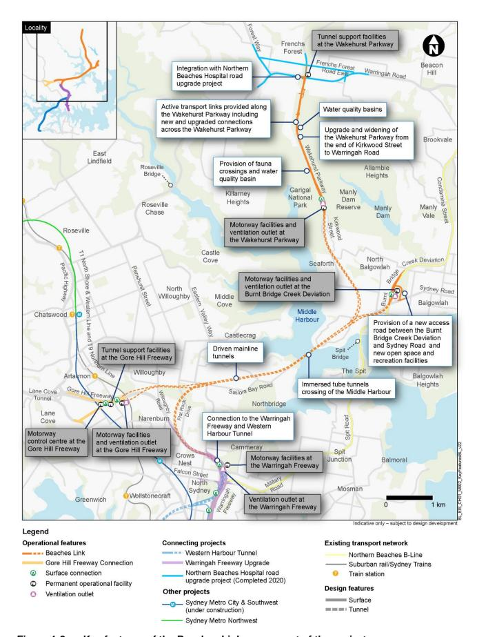
Figure 1-2 Key features of the Beaches Link component of the project
