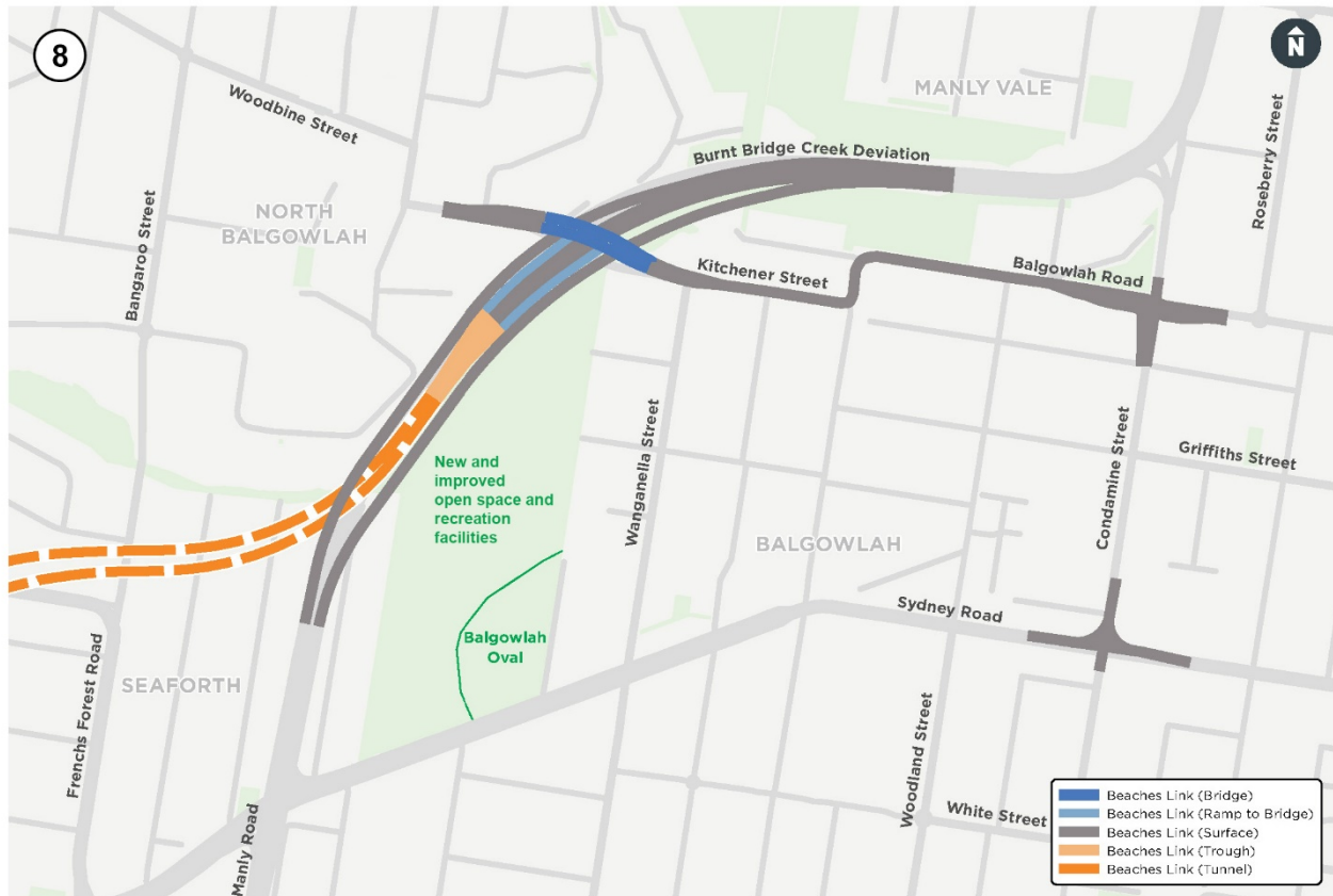
Figure 4-31 Alternative 8 - North facing tunnel ramps and surface ramps to Kitchener Street
