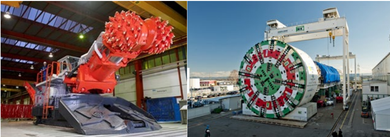
Figure 4-14 Examples of a roadheader (left) and tunnel boring machine (right)
