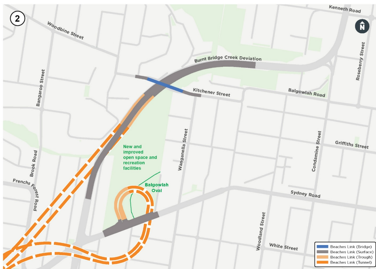
Figure 4-23 Alternative 2 - Tunnel loop ramps to Sydney Road
