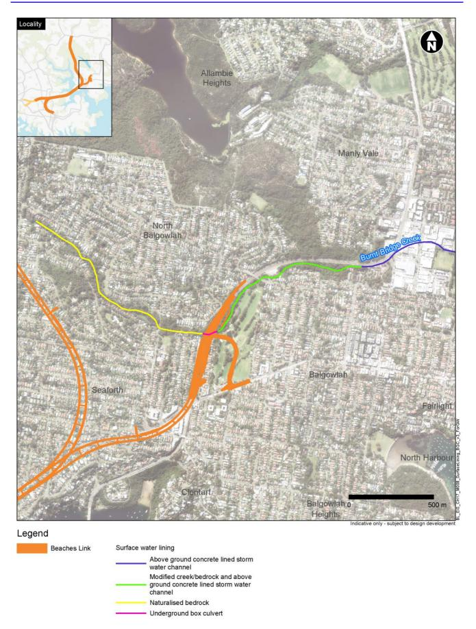
Figure 5-5 Surface lining of Burnt Bridge Creek
