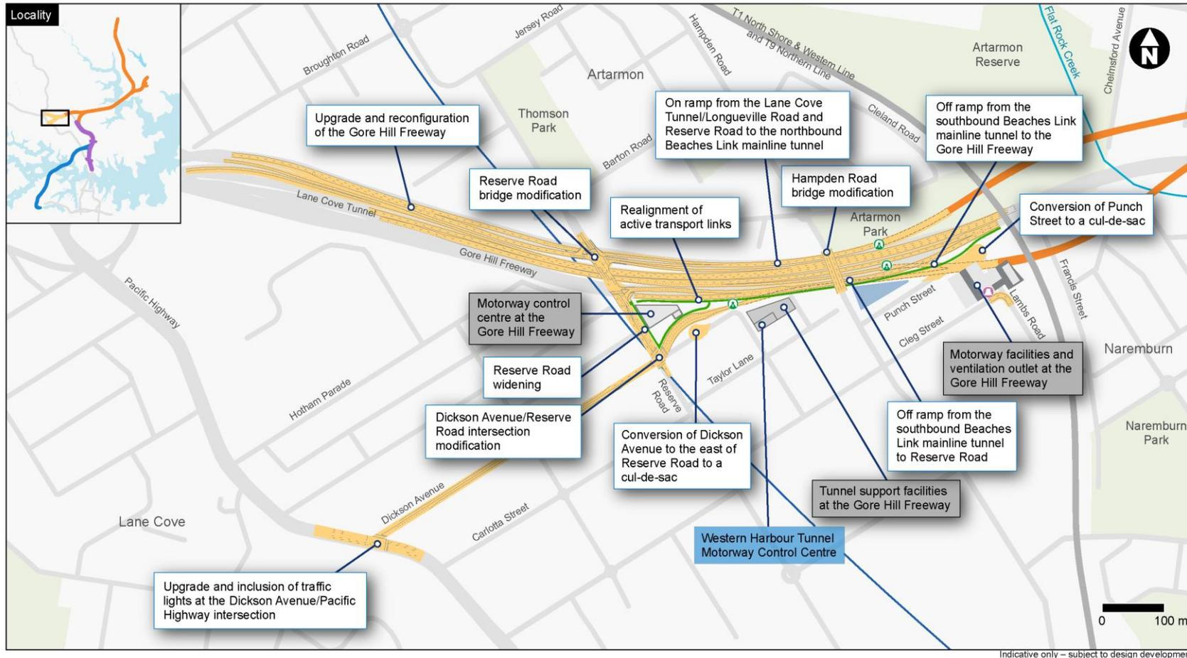
Figure 1-2 Key features of the Gore Hill Freeway component of the project
