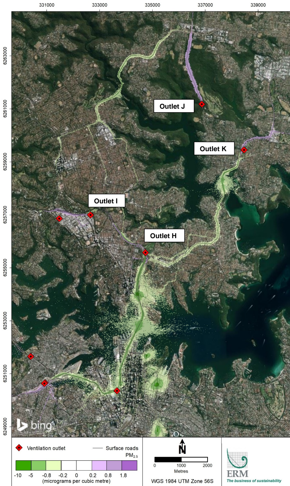
Figure 8-65 Contour plot of change in annual mean PM 2.5 concentration in the 2037 cumulative scenario (2037-DSC minus 2037-DM)
