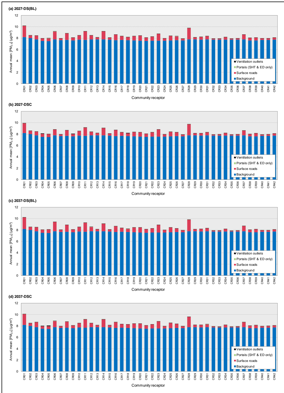
Figure 8-60 Source contributions to annual mean PM_{2.5} concentration at community receptors (with-project and cumulative scenarios) (portals include Sydney Harbour Tunnel and Eastern Distributor only)
