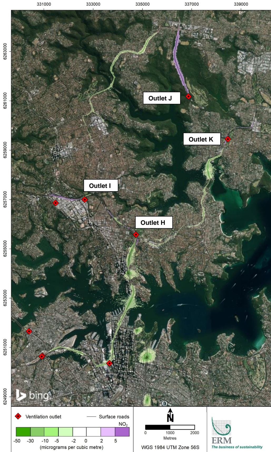
Figure 8-31 Contour plot of change in annual mean NO 2 concentration in the 2037 cumulative scenario (2037-DSC minus 2037-DM)
