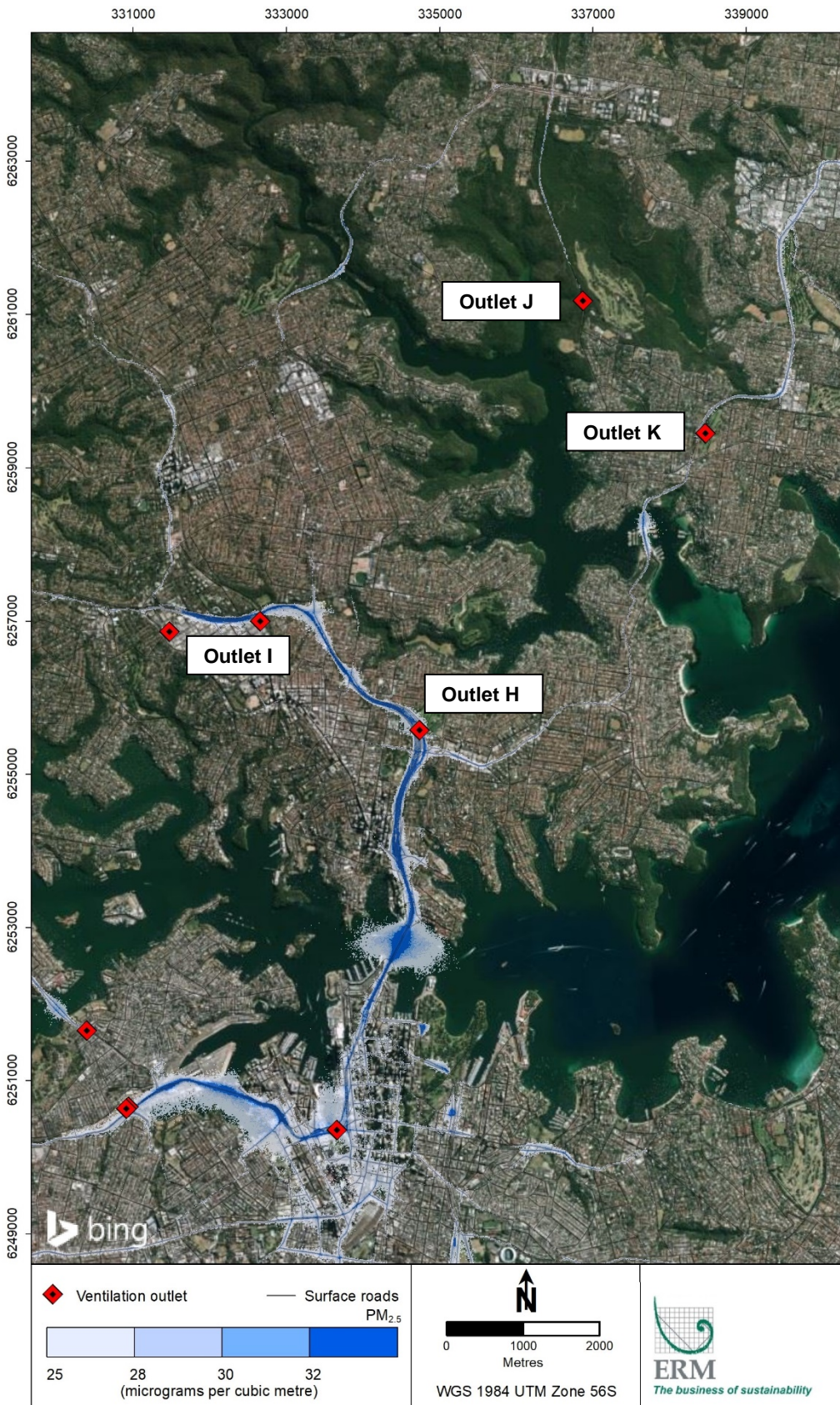
Figure 8-74 Contour plot of maximum 24-hour average PM_{2.5} concentration in the 2037 cumulative scenario (2037-DSC)
