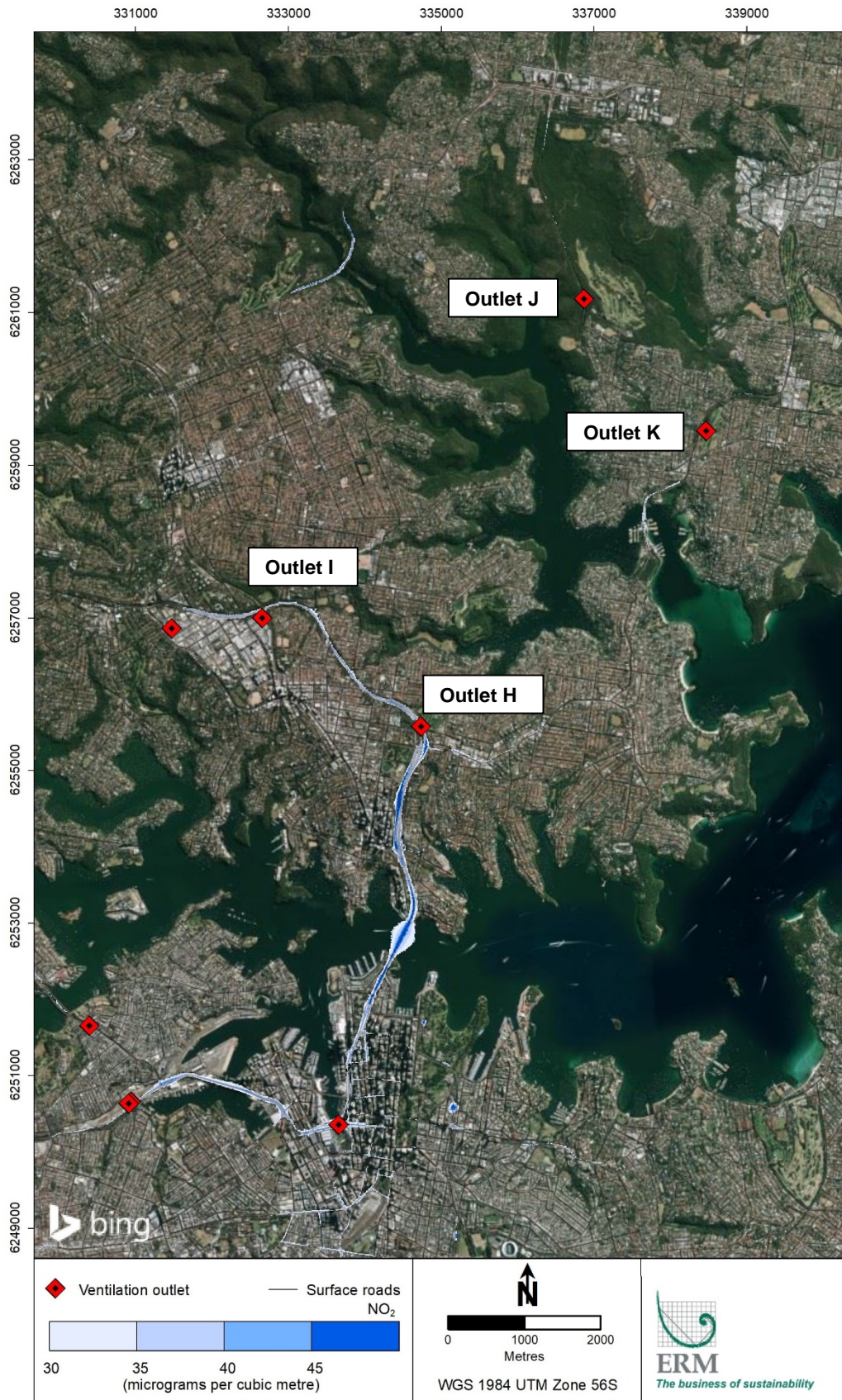
Figure 8-30 Contour plot of annual mean NO 2 concentration in the 2037 cumulative scenario (2037-DSC)
