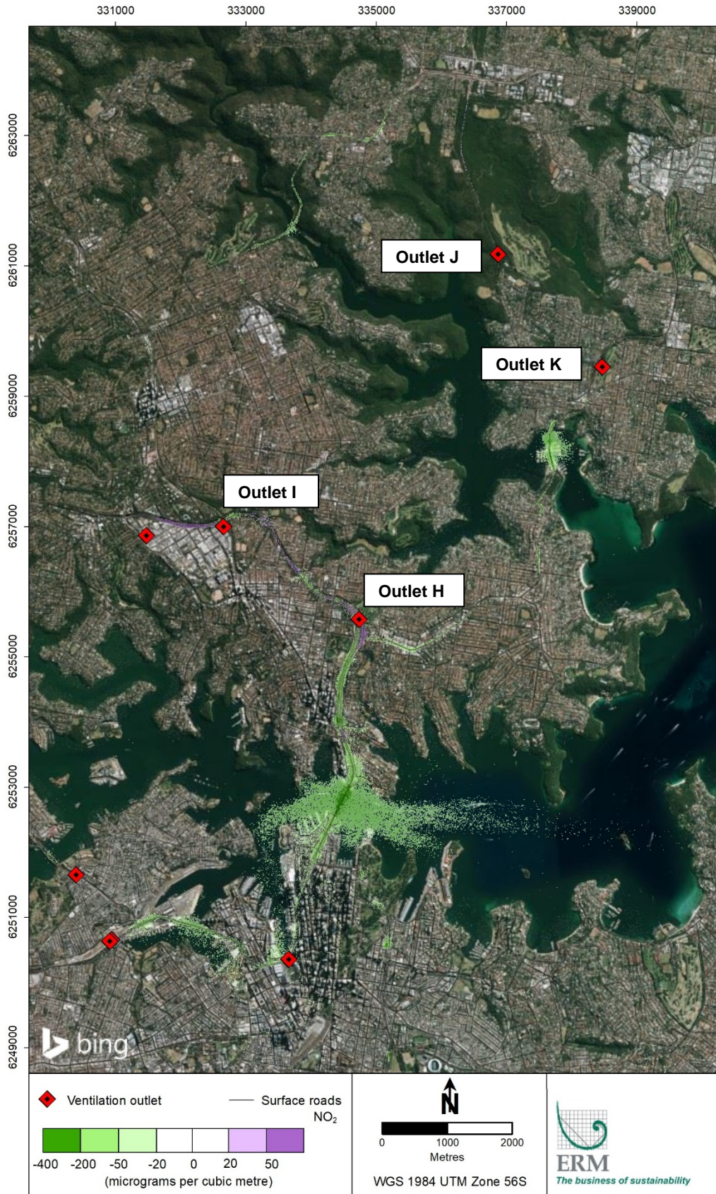
Figure 8-39 Contour plot of change in maximum 1-hour NO 2 concentration in the 2037 cumulative scenario (2037-DSC minus 2037-DM)
