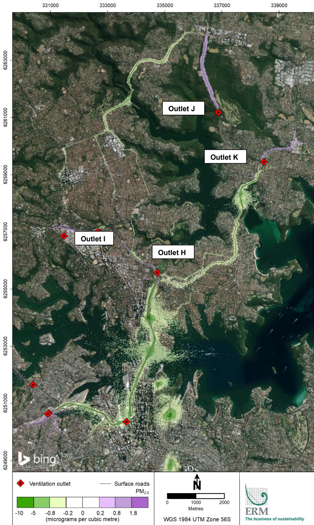
Figure 5-7 Contour plot showing change in annual average PM 2.5 concentrations associated with the project in the 'Do something cumulative 2037' scenario
