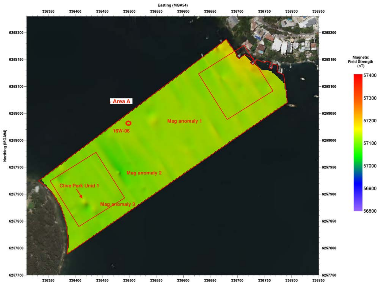
Figure 4-31: Magnetic anomalies in Area A (Earth Technology Solution Pty Ltd, July 2017b: Figure MH9A ). Target 16W-06 has been included to show that it displayed no magnetic signature, which means there is little ferrous content associated with it. The red boxes show the area of interest around the proposed cofferdams.
