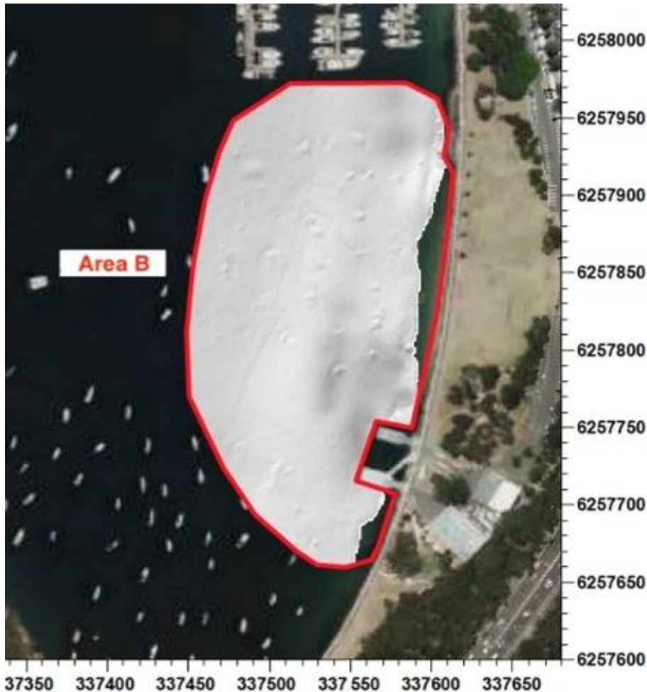
Figure 5-3: Bed of the harbour features derived from bathymetric survey within Area B (Earth Technology Solution Pty Ltd, July 2017a: Figure MH2A). Low circular mounds are moorings for recreational craft
