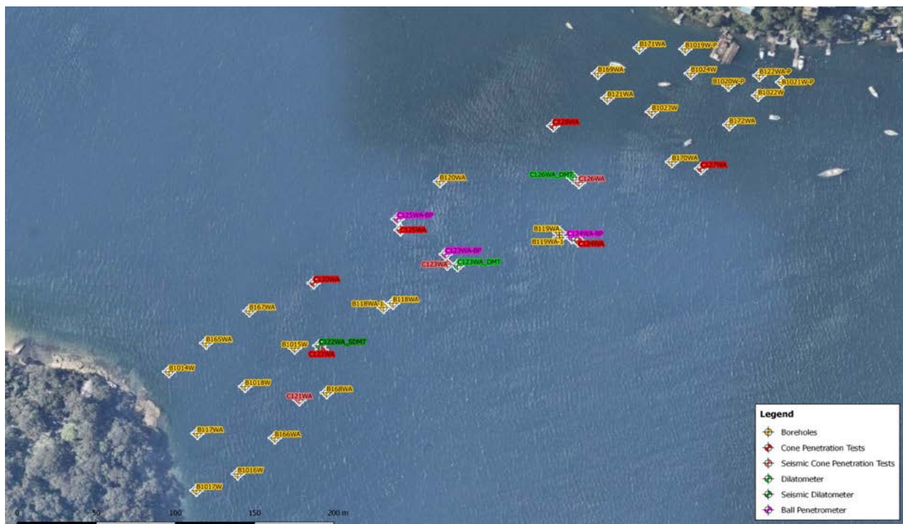
Figure 4 Drilling sites within Area A (Golder Associates and Douglas Partners, October 2017 Test Locations; Western Harbour Tunnel and Beaches Link; Middle Harbour. Drawing No. 2, Revision 1, drawn 19 October 2017).
