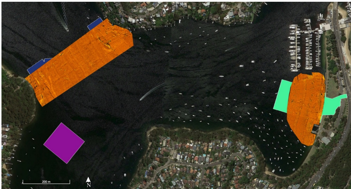
Figure 2: Extent of side scan sonar survey in relation to proposed extent of disturbance footprint (in solid blue and solid orange) (Base image: Google Earth). Side scan sonar data provided as .shp files by Podnar, A. Geotechnical Engineer, Douglas Partners, 5 December 2017.
