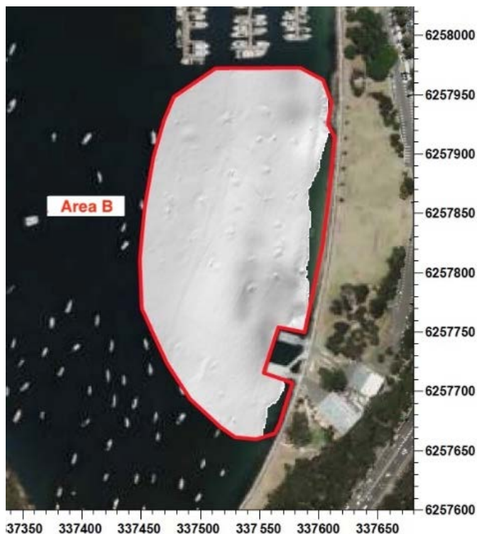
Figure 21 (left): Bed of the harbour features derived from bathymetric survey within Area B (Earth Technology Solution Pty Ltd, July 2017a: Figure MH2A). Low circular mounds are moorings for recreational craft.
