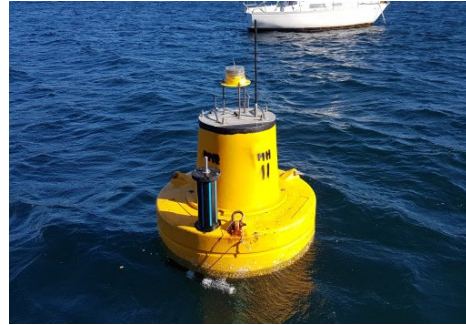
Aquadopp Z-Cell mounted underneath buoy at MH2
