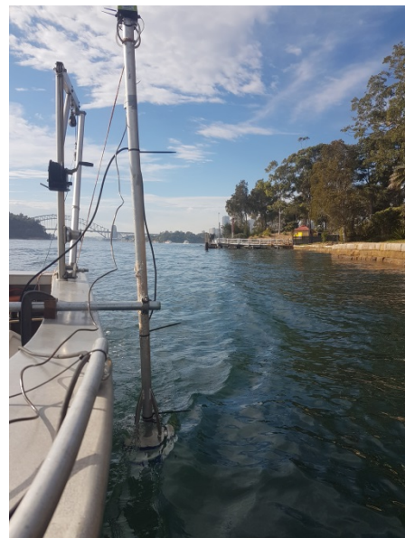
Vessel mounted ADCP transect setup
