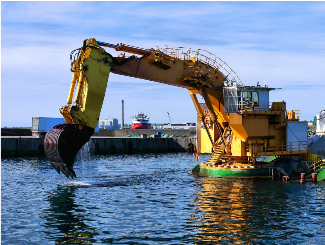
Figure 7-2: Example of a very large backhoe dredge operating with standard open bucket attachment
