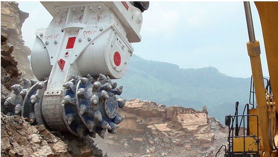
Figure 7-4: Example of drum cutter attachment on an excavator stick
