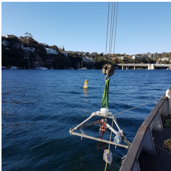
Bottom mounted ADCP during deployment at MH1
