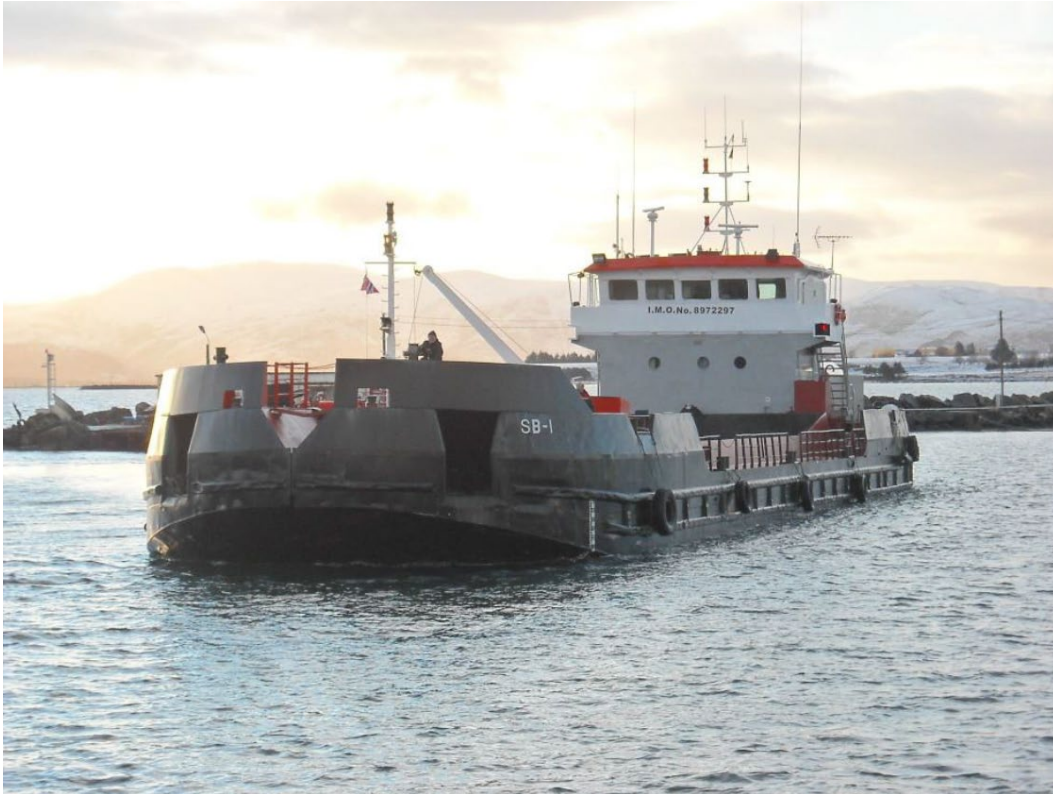
Figure 7-3: Example of self-propelled split hopper barge
