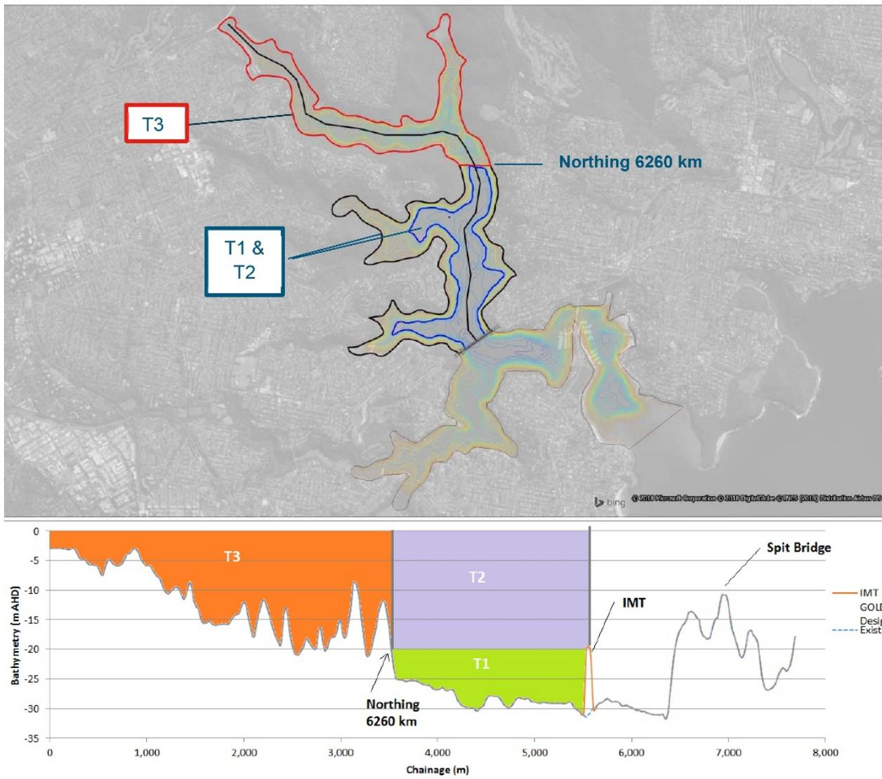
Figure C-3 Waterbodies upstream of the crossing (above) and long section of Middle Harbour (below) (Source: Appendix P (Technical working paper: Hydrodynamic and dredge plume modelling))
