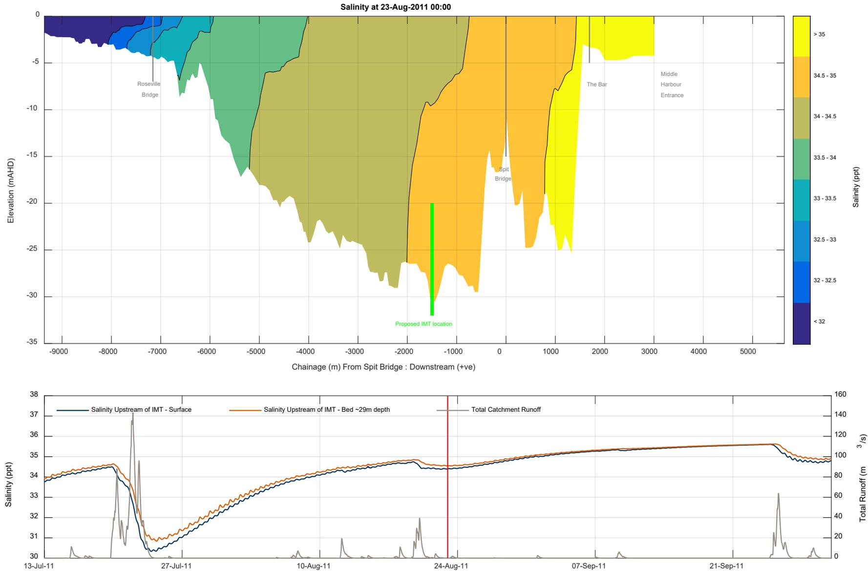
Figure 3-5 SHERM high resolution water quality model salinity results (reproduced from LLS)
