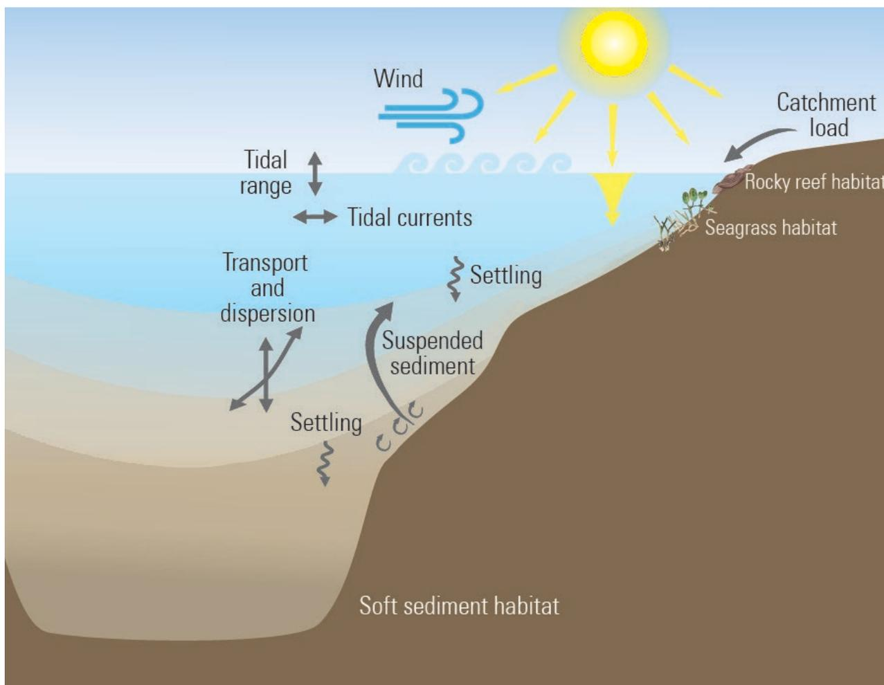
Figure 3-2 Water quality processes schematic
