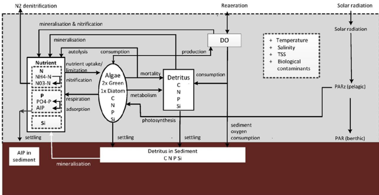
Figure C-2 Water quality processes in the SHERM (WAQ) module (after Deltares, 2011)
