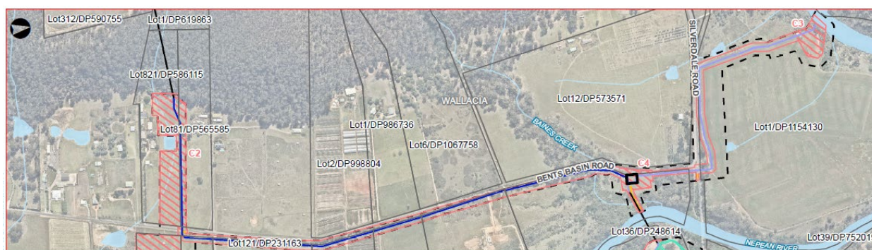
Plate 1.5 Environmental flows pipeline alignment going south along Bents Basin Road before turning west and under-boring to a release point at Warragamba
