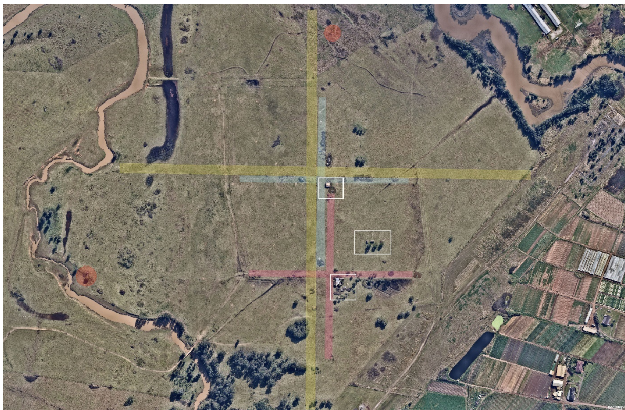
Figure 48. Indicative site plan of Fleurs Field Station with Parabolic Antennae shaded in red, Mills Cross shaded in blue, Chris Cross shaded in pink and the Shain Cross shaded in yellow. The buildings are located within the white boxes.
