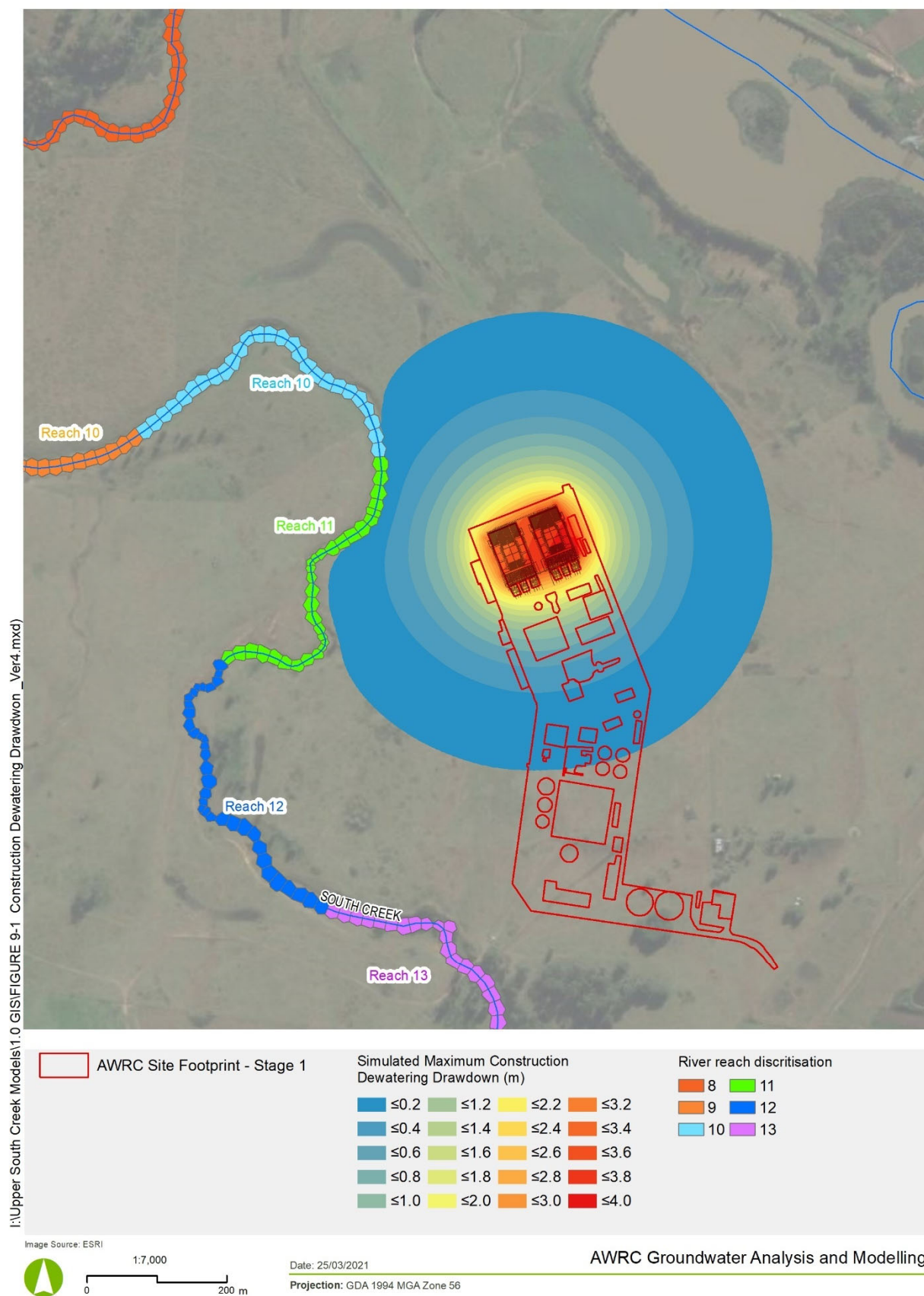
Figure 7-2: Construction Dewatering Drawdown (Cone of Depression)
