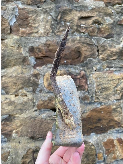
Figure 4-35: Example of metal bracket from timber beams with a long, handmade nail.
