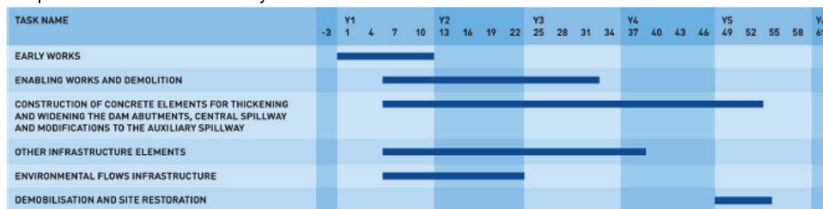
Figure 2-2: Preliminary construction program
