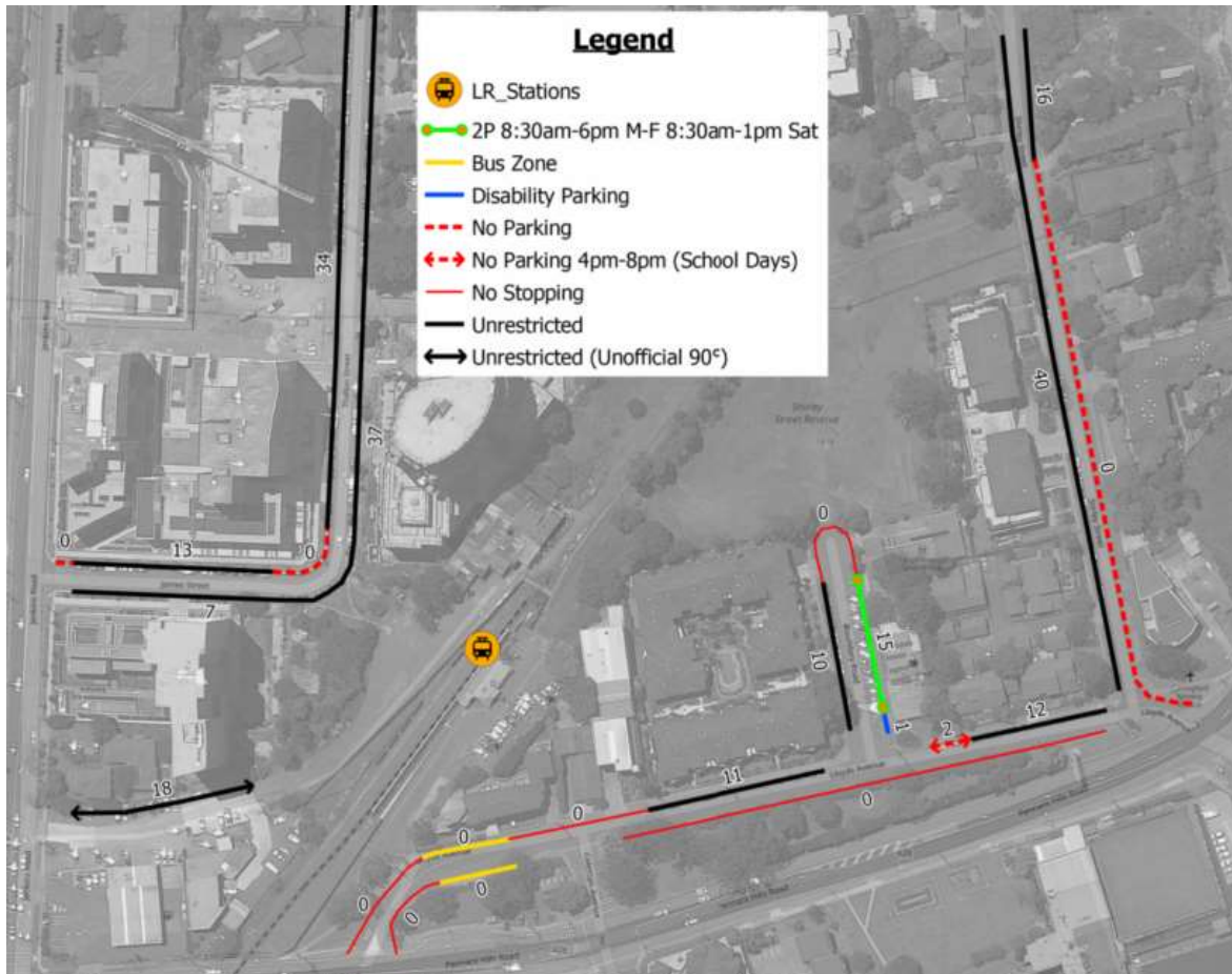
Figure 3.83: Carlingford Station – Existing Parking Conditions
