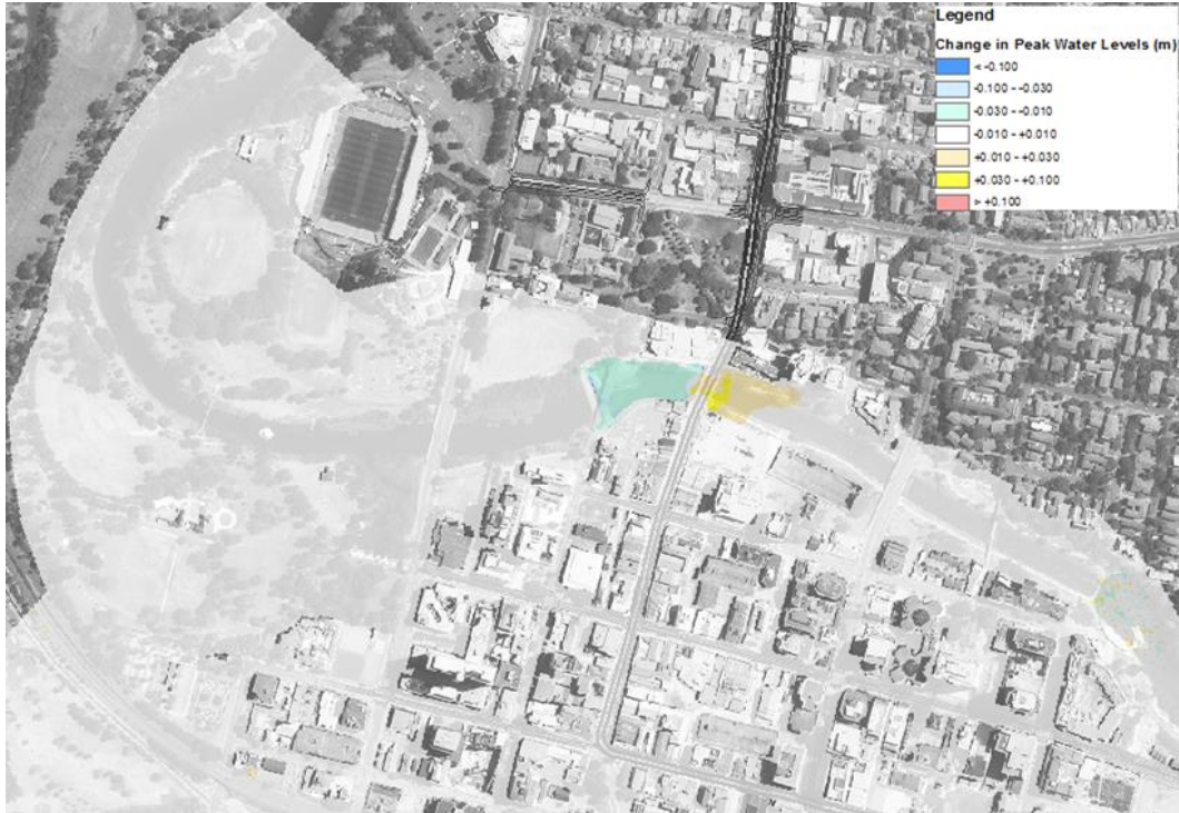
Figure 31 Change in Peak Water Levels with Lennox Bridge Bikeway Portals - 0.2EY Event
