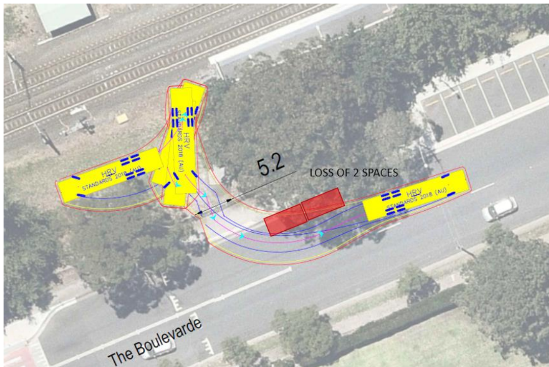
Figure 4.14 – WP2 – M24 15.440D Parking Space Loss
